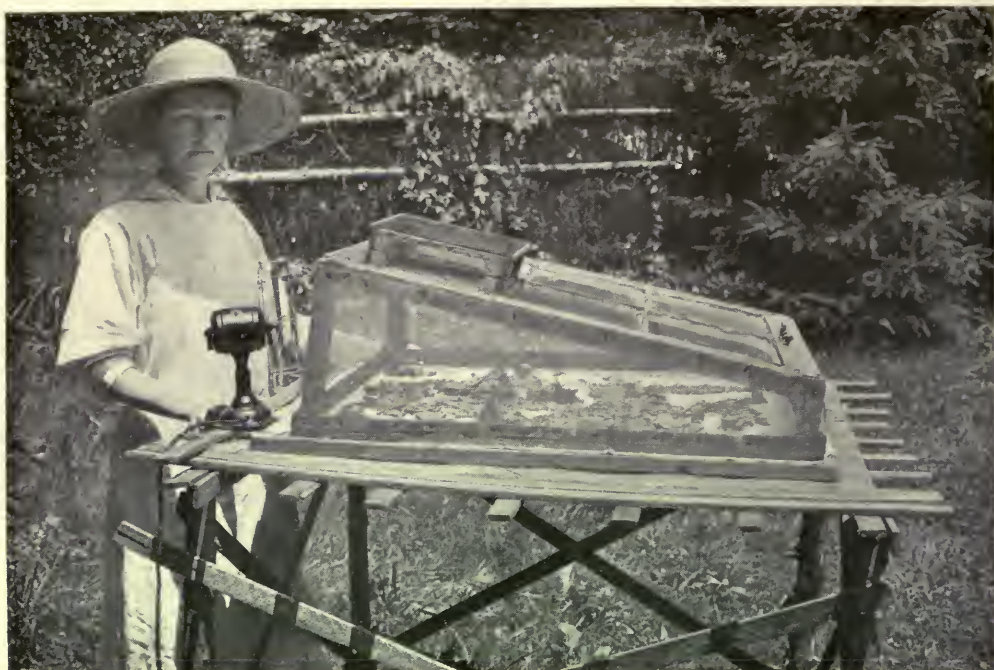
AN INEXPENSIVE SUN DRIER MADE OF ONE WINDOW SASH, A FEW LATHS, AND SOME METAL FLY SCREEN
