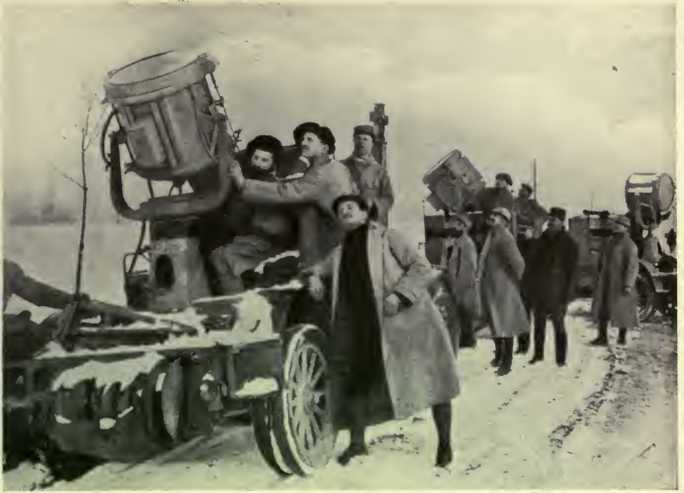
THE AUTOMOBILE SEARCHLIGHTS WHICH ARE MOST EFFECTIVE IN SEARCHING OUT THE ENEMY'S ZEPPELINS, THUS AIDING IN BRINGING THEM DOWN
