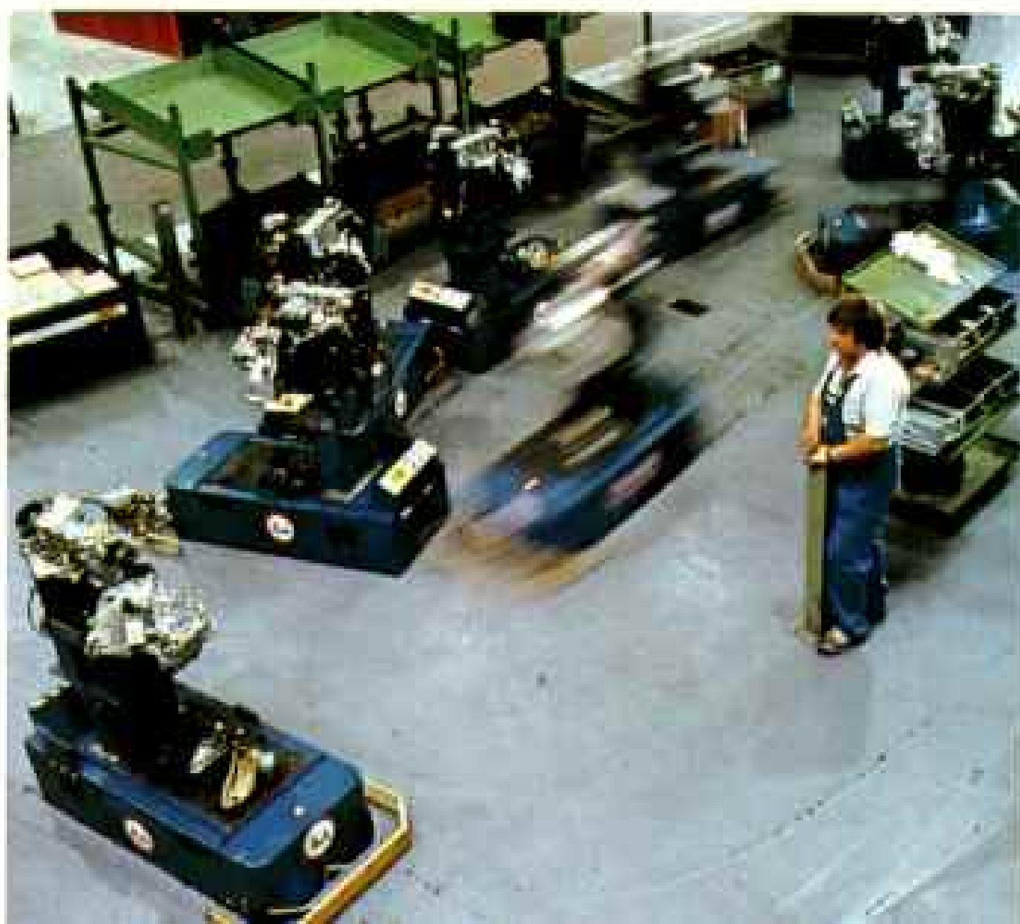
Robot express, guided by induction wires embedded in the floor (right), trundles engine blocks on demand to workers who mate them to transmissions at the Vienna General Motors plant, completed in 1982.
