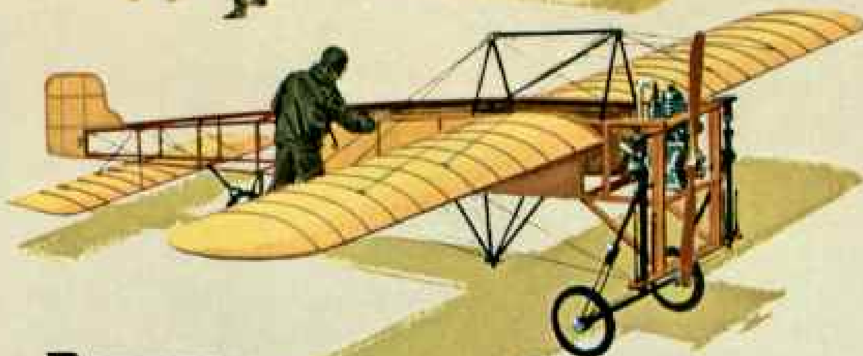
Louis Blériot's Type XI used a single wing, box-girder fuselage, control column, and rudder bar. In 1909 Blériot was first to fly the English Channel, a preview of the practical uses of the airplane.
