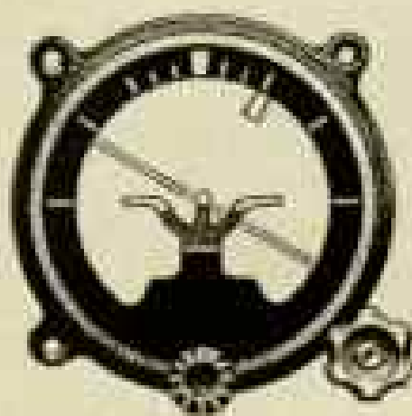
Gyrosopic artificial horizon, new in 1929, permitted true blind flight. This one from the 1940s shows a left turn.
