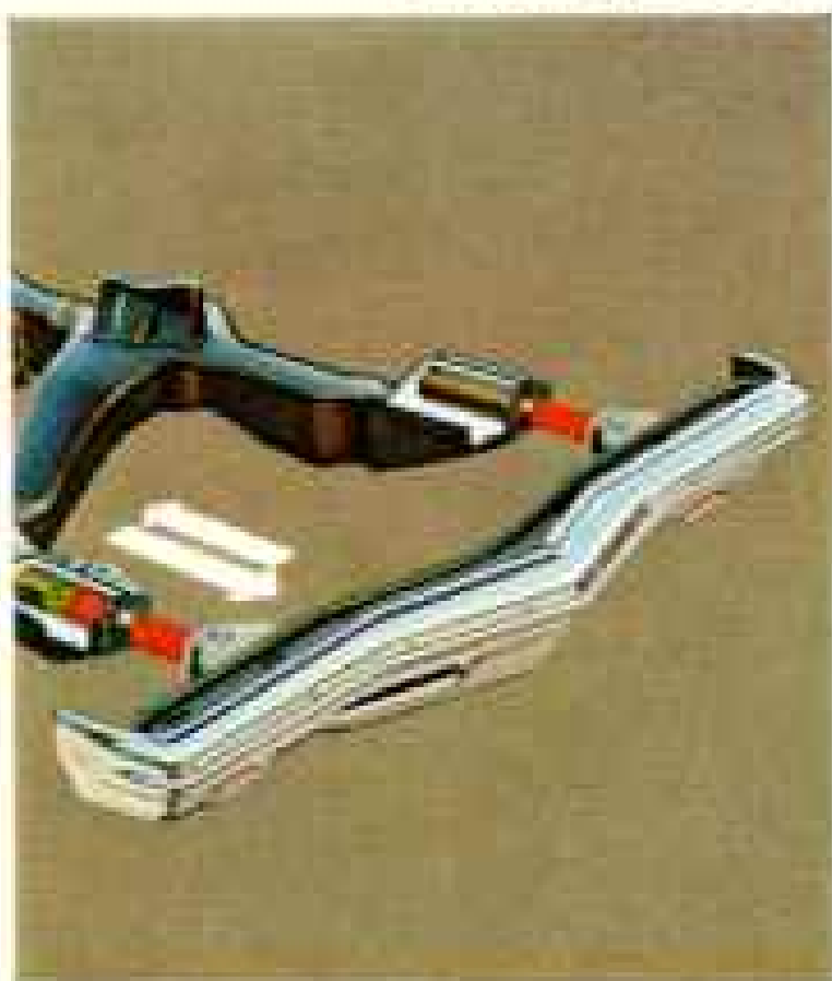
Impala’s front bumper system recoils hydraulically on minor impact to help cushion shocks.
