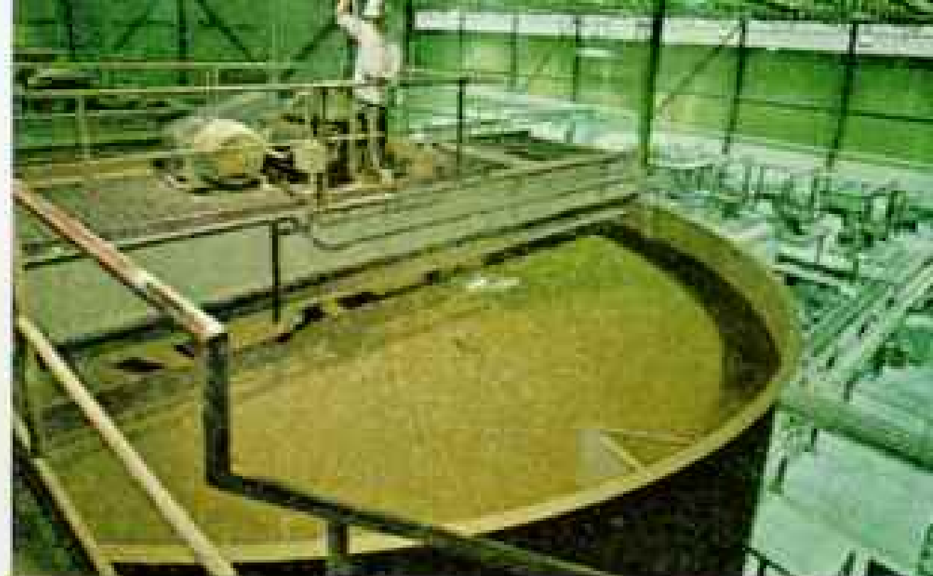
Agitator tank concocts a soup of finely ground ore and powerful cyanide solution used to dissolve gold.
