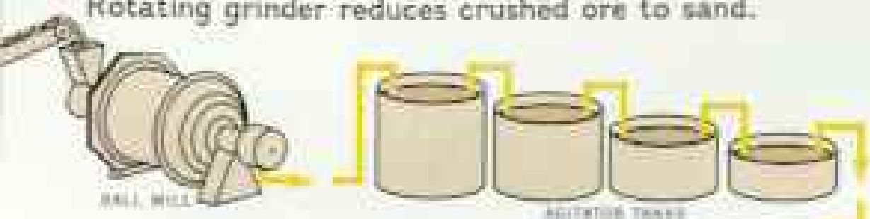
Rotating grinder reduces crushed ore to sand.
