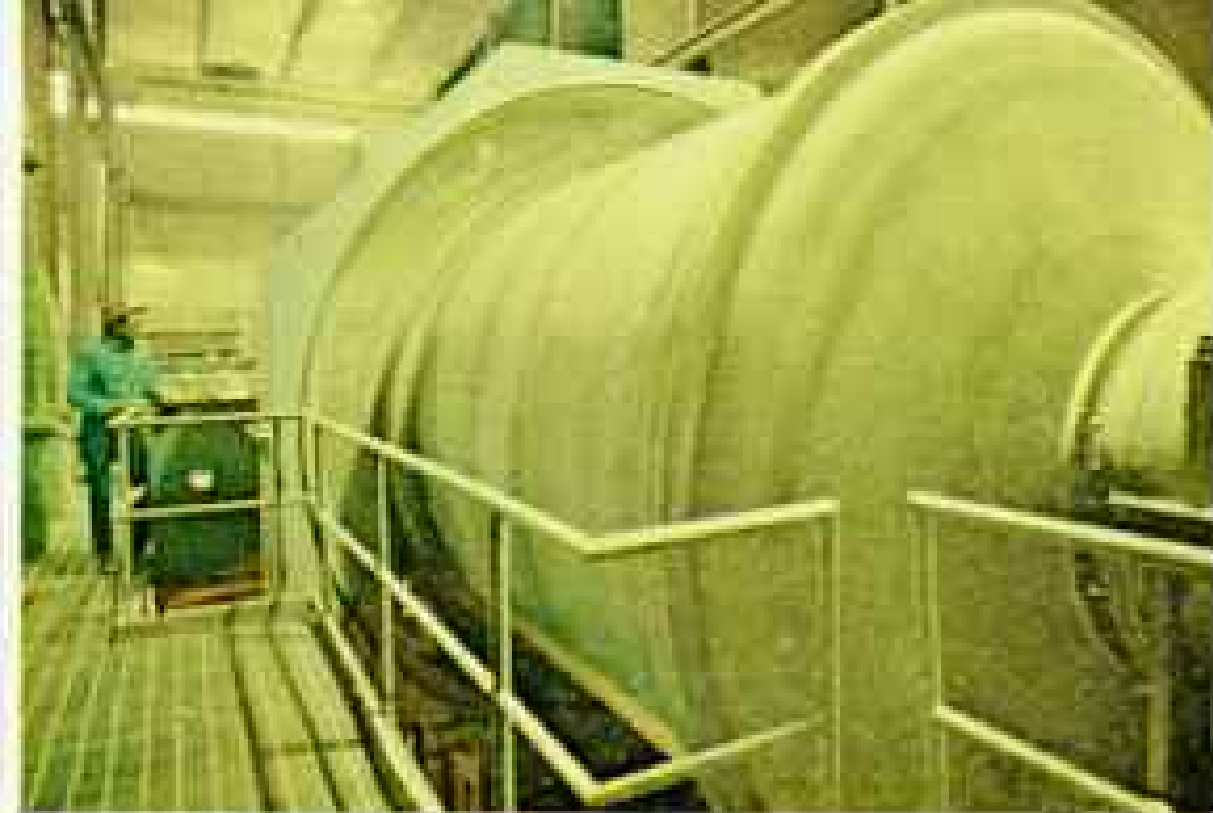
Rotating grinder reduces crushed ore to sand.
