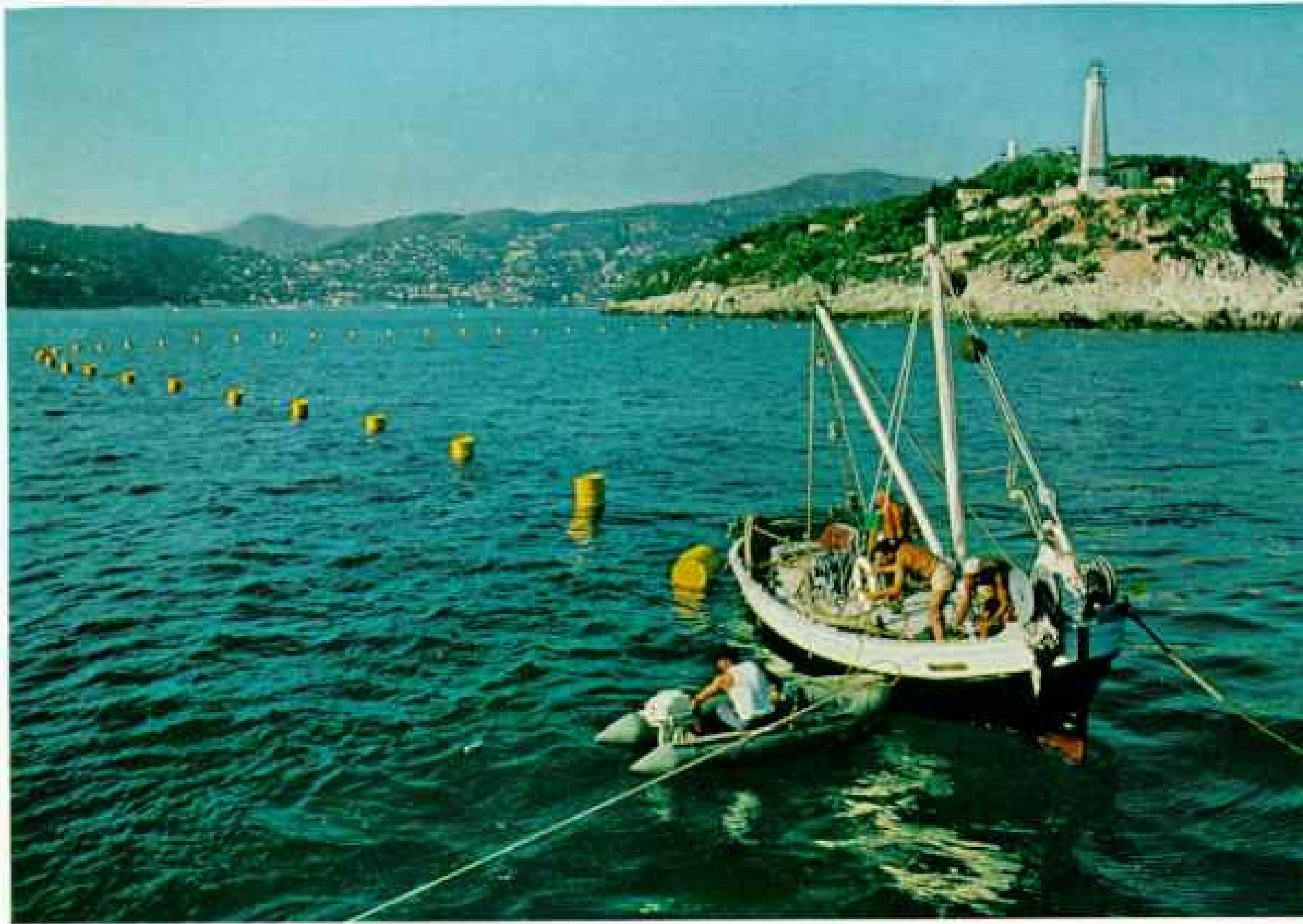
Half-mile arc of buoys, holding up power and communication lines, links the diving site with Cousteau's headquarters in the Cap Ferrat lighthouse. Line to left helps the research boat Physalie fight the current as her crew awaits Conshelf Three's descent.
