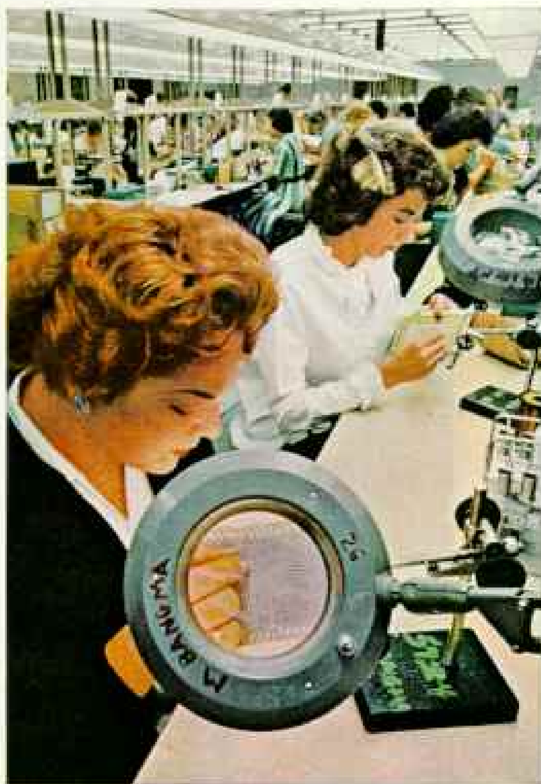
Wire weavers shape memory units for computers at a Litton Industries plant in Woodland Hills.
