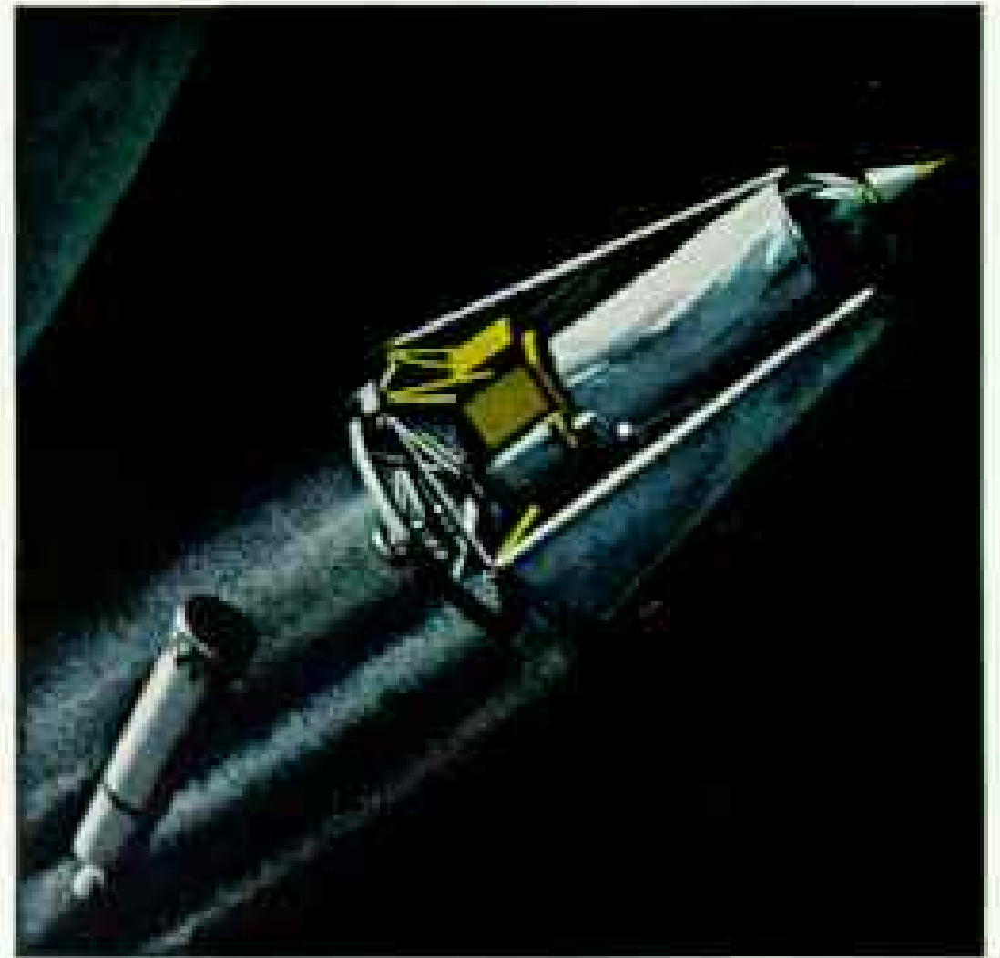
3. Spent Agena, parted from Ranger by springs, falls away. A retrorocket will take the glittering Agena away from Ranger's light-seeking devices.
