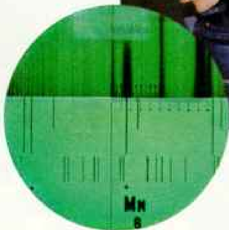
Spectrographic test (above) of particles from wreck shows manganese (Mn, left) from a battery.
