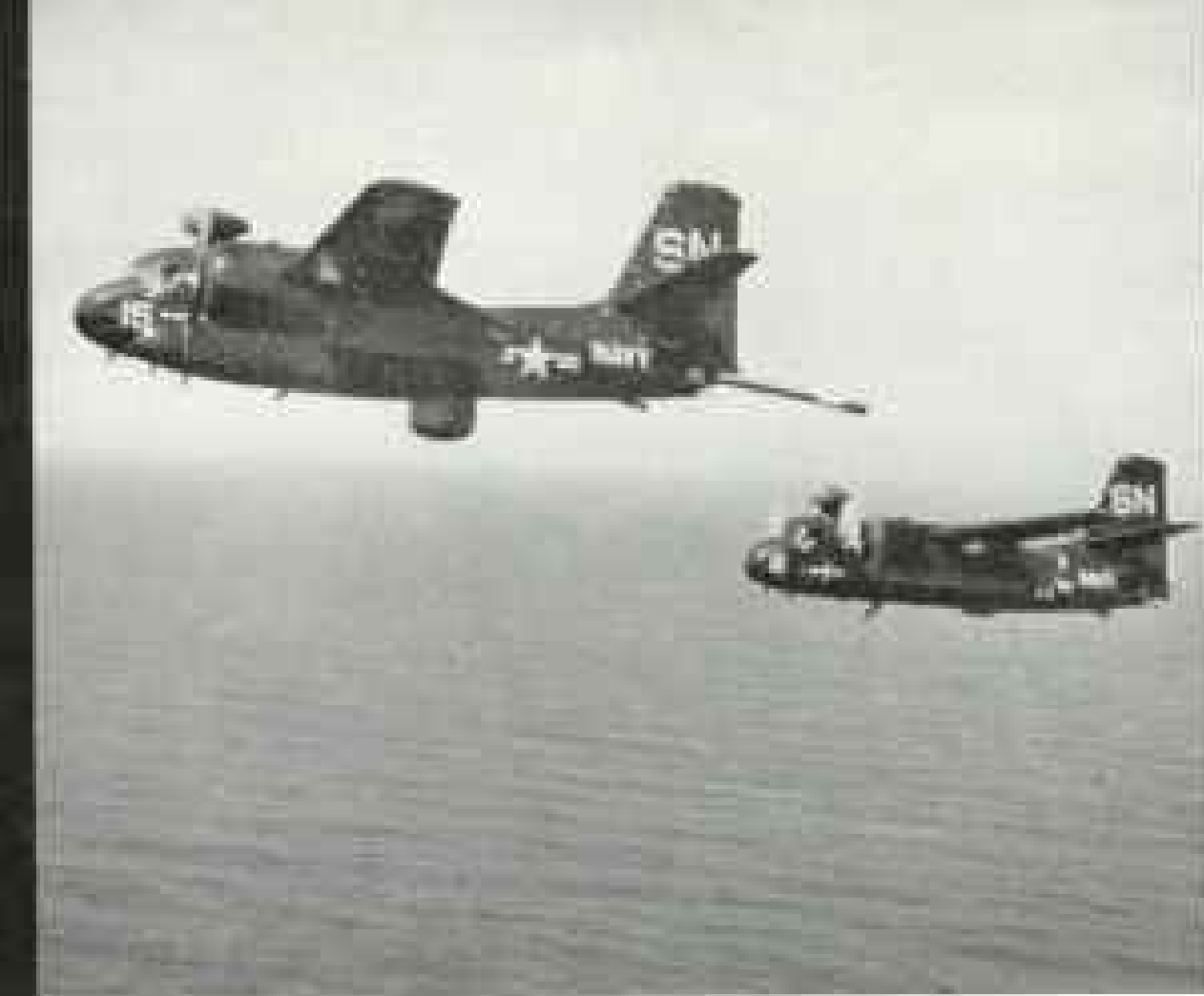
1618. Grumman S2F's start search with electronic gear that can detect snorkel, periscope, or sub radar, even the submerged sub's disturbance of the earth's magnetic field.
