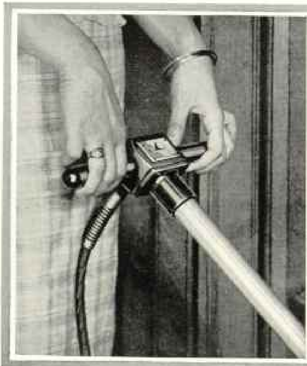
No strength is needed to operate the machine. You guide it by raising or lowering the handle
