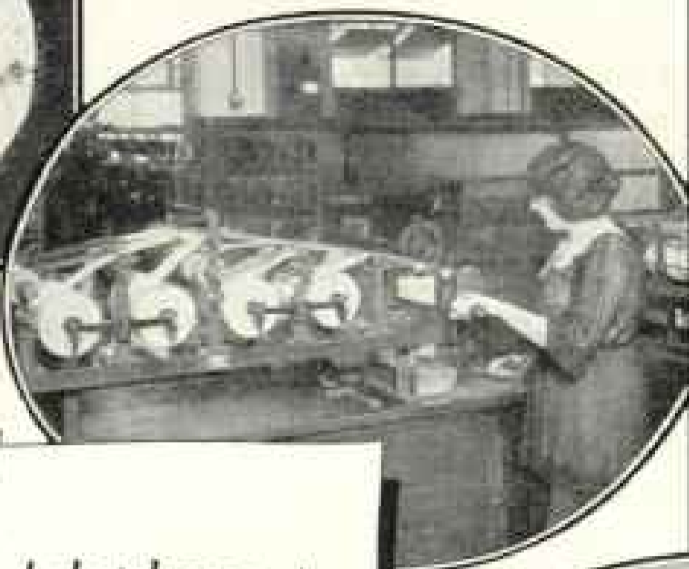
Winding the telephone condenser, from linen paper and tin foil. The condenser keeps electric currents where they belong.
