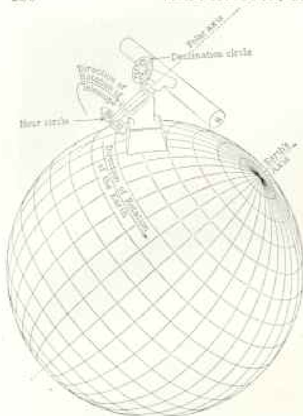
DIAGRAM SHOWING THE USUAL METHOD OF MOUNTING A BIG TELESCOPE
