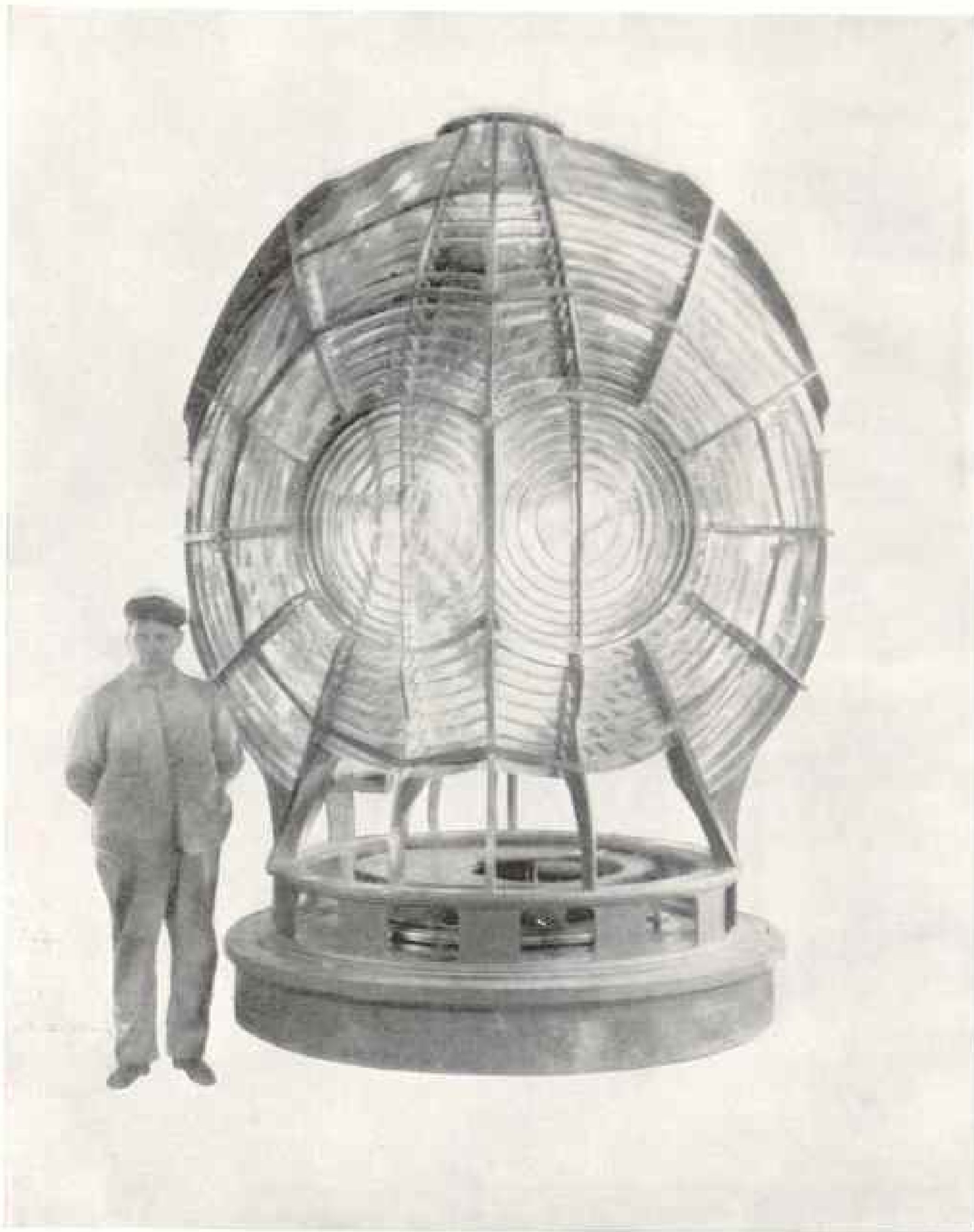
A BEAUTIFUL GLASS LENS AND MOUNTING RECENTLY BUILT IN FRANCE FOR THE KILAUEA LIGHTHOUSE NOW UNDER CONSTRUCTION IN THE HAWAIIAN ISLANDS
