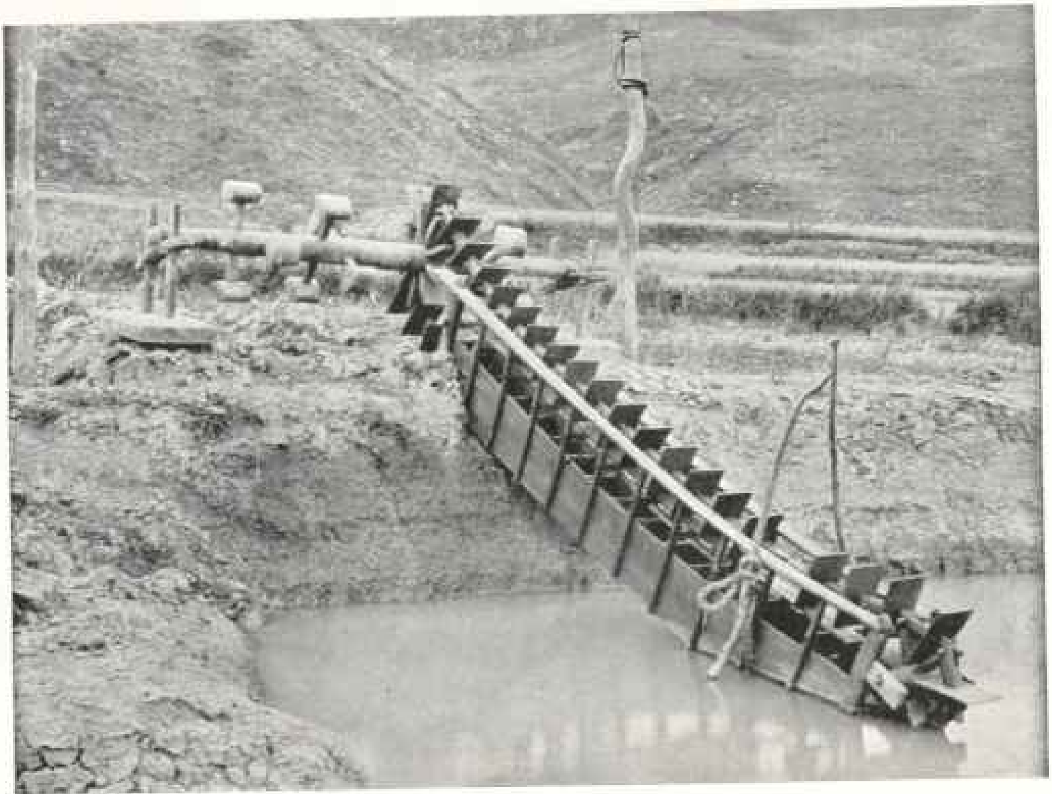
THREE-MAN CHINESE FOOT-POWER AND WOODEN CHAIN PUMP, EXTENSIVELY USED FOR IRRIGATION IN VARIOUS PARTS OF CHINA.
