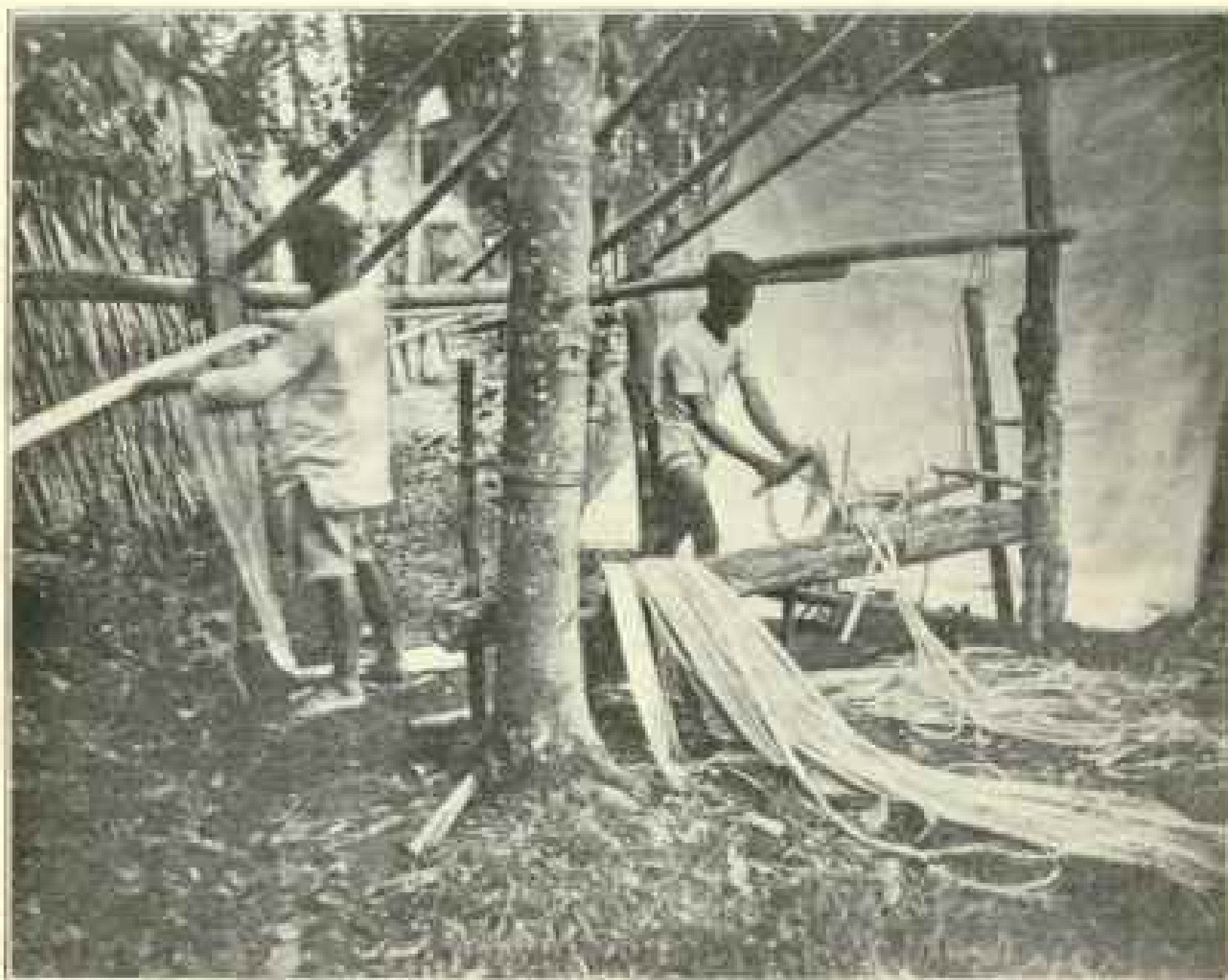
THE BAY STRIPS OF THE JUTEA TEXTILES AFTER BEING DRIVEN SEVERAL TIMES UNDER THE FEET
