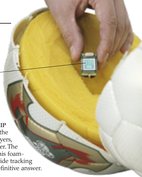
A microchip inside the ball will determine whether the ball crossed the line
