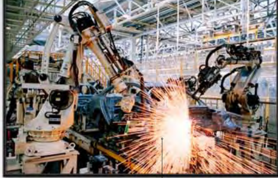
The task of welding in a car factory is carried out by robots
