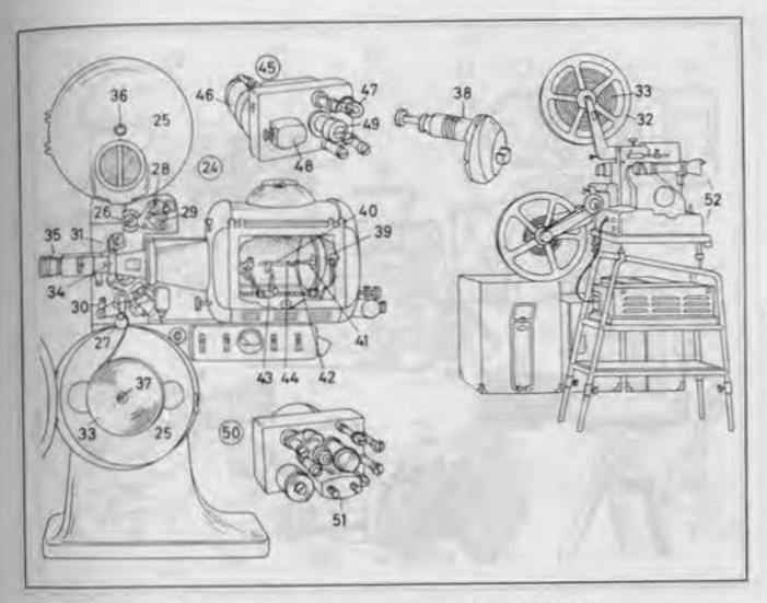
30 loop former for smoothing out the intermittent movement; also: film break detector
