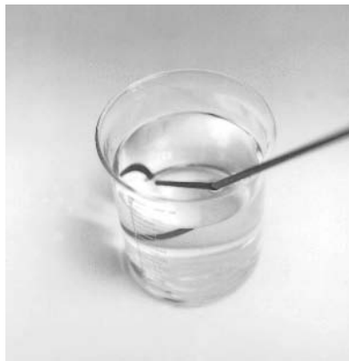
Fig. 6.6a,b. Photographs of a stirring rod in a beaker. Photograph (a) is of an empty beaker, and the glass rod appears straight. Photograph (b) is of a beaker partially filled with water. The rod appears to be bent at the water surface.
