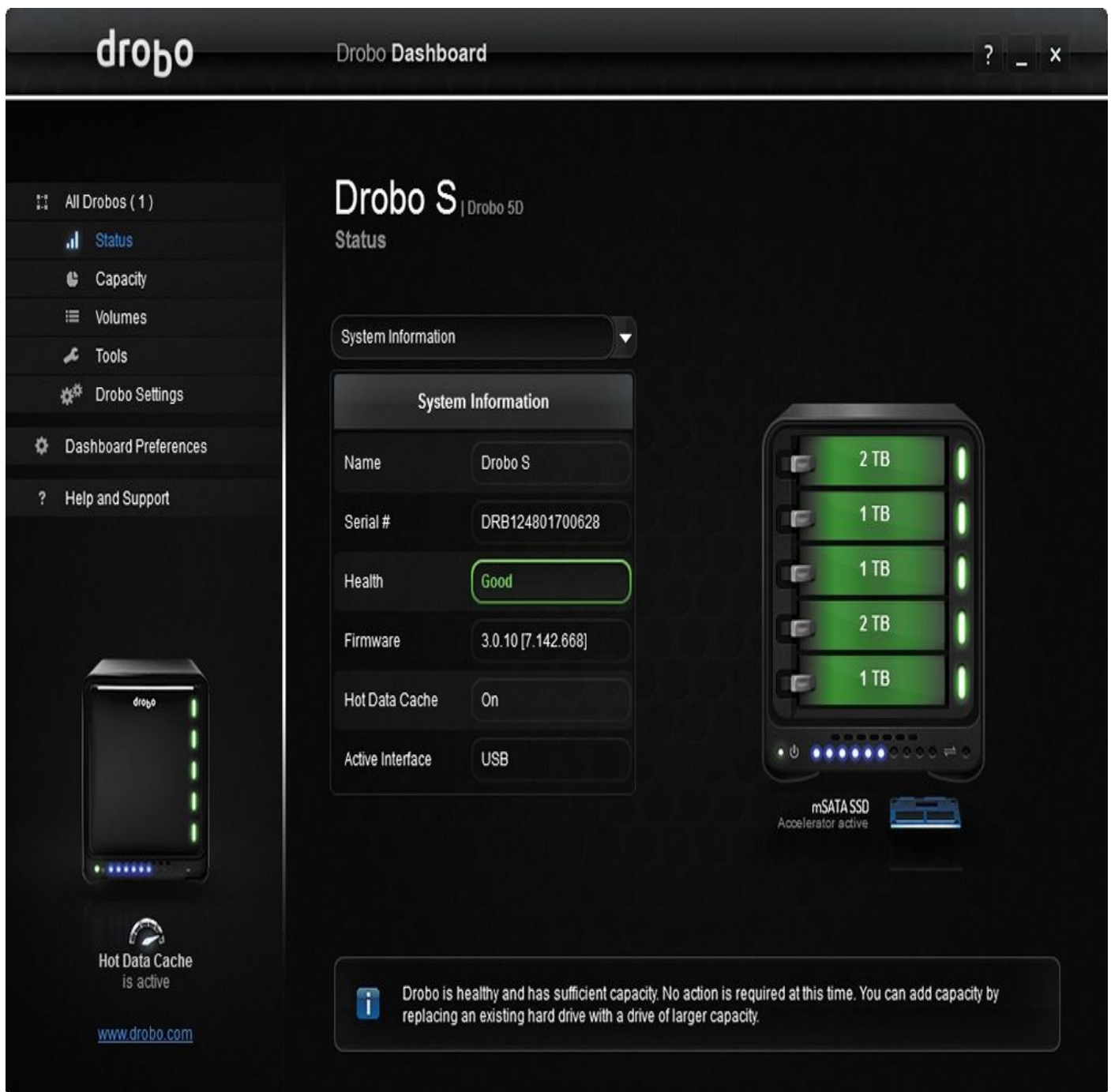
Figure 9.10 My Drobo contains five drives varying in size from 1 to 2 terabytes. As drives fail, I can replace them inexpensively and without any loss of my images.
