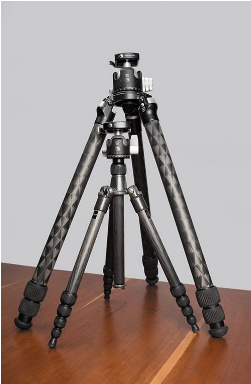
Figure 1.7 My larger tripod is much sturdier and a requirement when I need a tack-sharp landscape image. There's no use in using mirror lock-up (a feature on DSLRs that allows the mirror to be locked up to reduce vibration during exposure) and a shutter release if your tripod wiggles in the wind. On the other hand, if I need lightweight and small for foot travel, I use the travel tripod.
