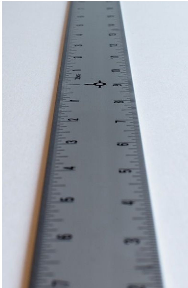
Figure 3.13 A narrow aperture such as f/10 creates a deeper depth of field.
