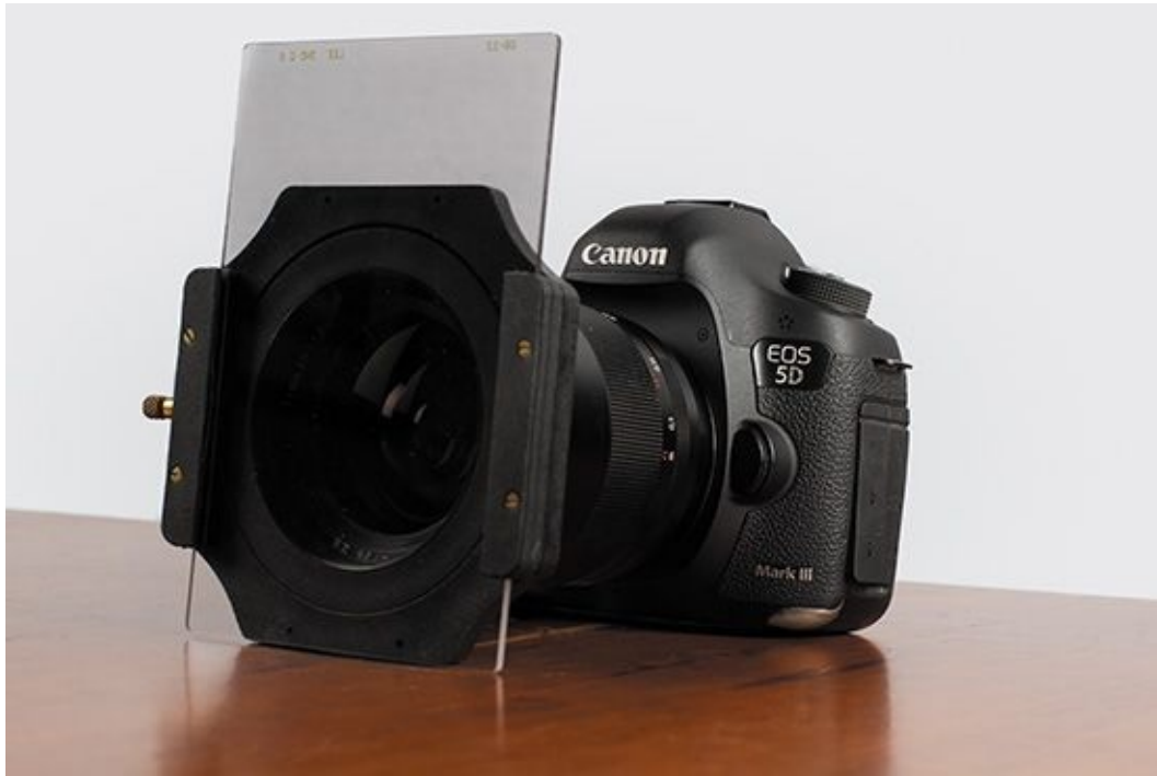
Figure 1.10 A graduated ND filter is a must if you want to create long exposures during the bright daylight.
