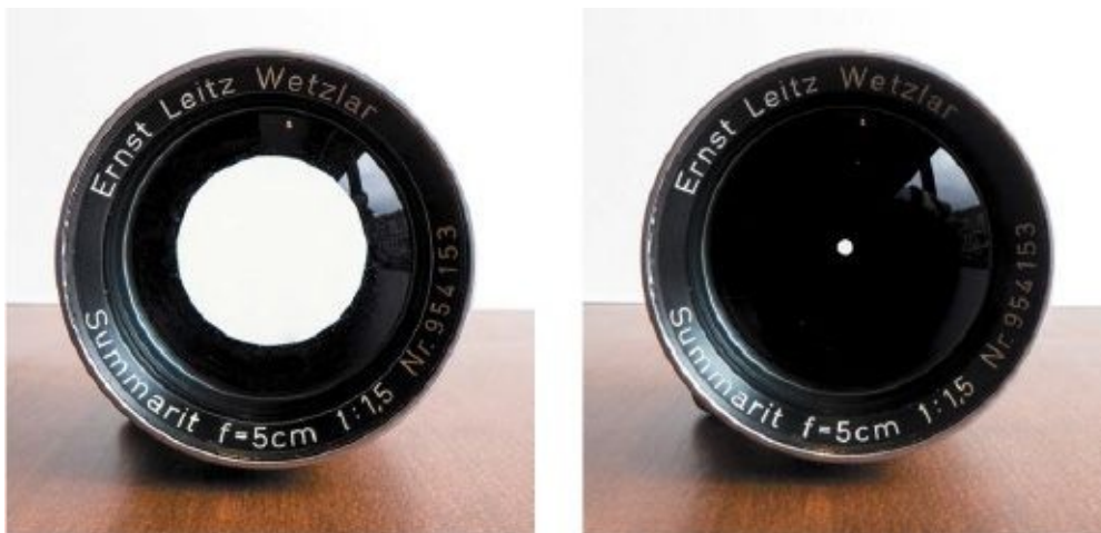
Figure 3.10 The lens on the left has a much wider aperture of f/1.4 than the lens on the right, which has an aperture of f/16.
