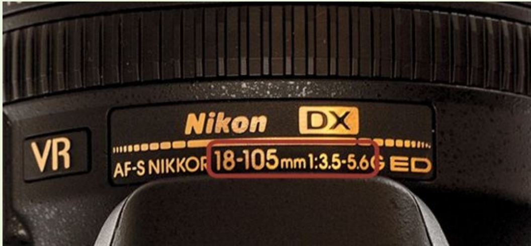
Figure 3.11 Nearly all zoom lenses are marked with the widest aperture for a given focal range.
