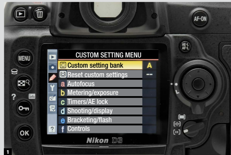
1 A custom settings bank is a location where you can store your personal selection of important settings, for rapid access.
