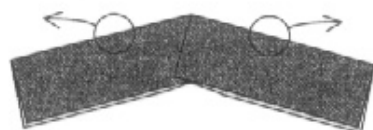
1. Example of a stretched pleat. Pull the two sides apart, keeping the angle fixed.
