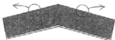
1. Example of a stretched crimp. Pull the two sides apart, keeping the angle fixed.
