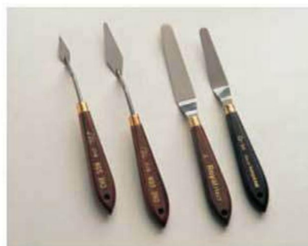
Knives The knives on the left are painting knives; those on the right are palette knives. The steep angle in the neck of painting knives keeps your hand from getting in the paint.
