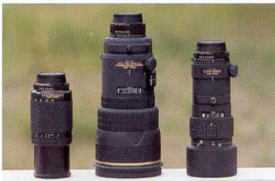
These three 300mm lenses demonstrate the difference that maximum aperture makes. From left to right: a 70–300mm f/4 –5.6 zoom lens set at its 300mm length; a 300mm f/2.8 lens; and a 300mm f/4 lens. I have not added a lens hood to any of these in order to show their actual size differences.
