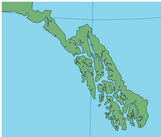
The State Plane Coordinate System uses Hotine Azimuth Natural Origin for the Alaskan panhandle.
