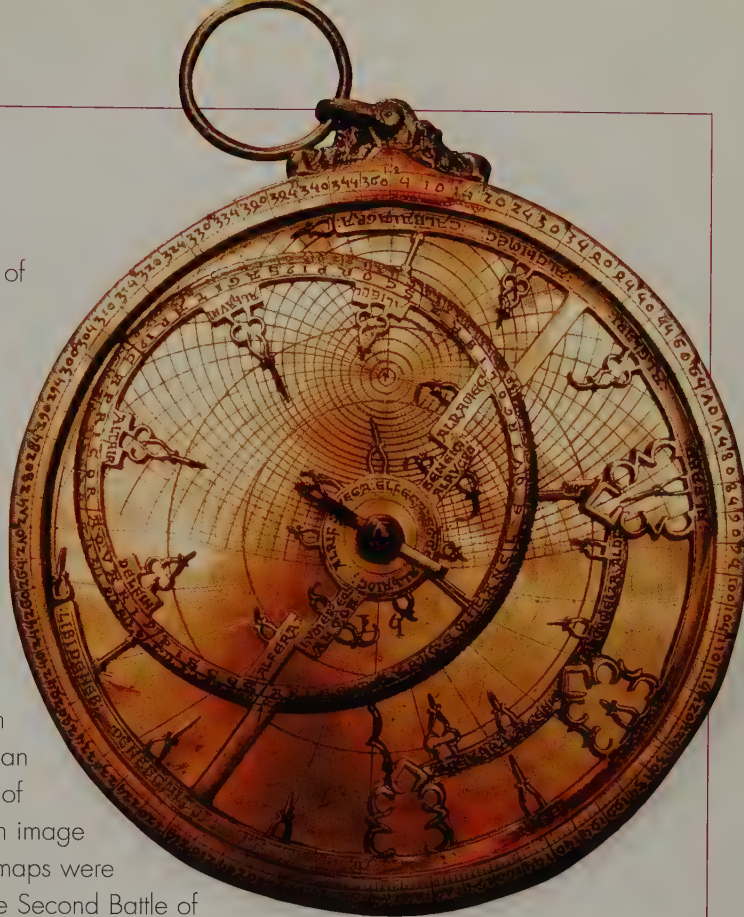
Above: A 13th-century astrolabe, used to take altitude measurements of the sun or a star for finding latitude. Astrolabes have been in existence for over a thousand years. They were popular in Europe between the 15th and 18th centuries, after which a new generation of astronomical instruments, such as the telescope, began to emerge.
