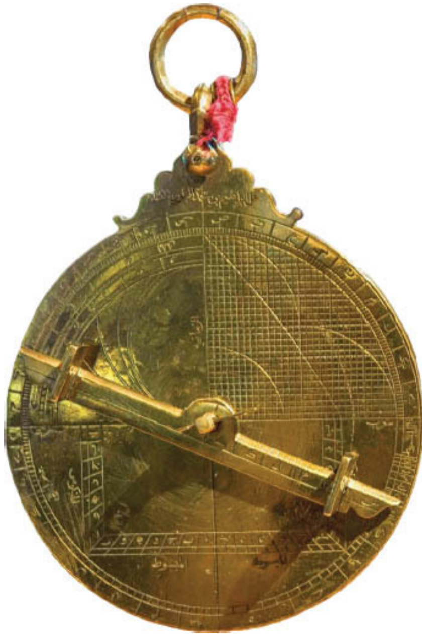
The face of an astrolabe with the rete clipped to its surface; and on the reverse the alidade and various notched rules of measurement.
