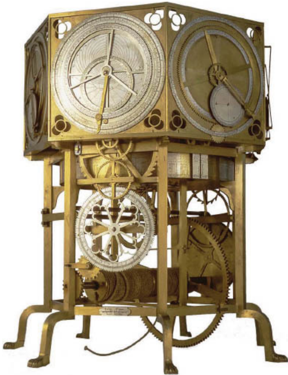
A mid-twentieth century reconstruction of de Dondi's famous astrarium, a mechanical realization of the Ptolemaic universe.
