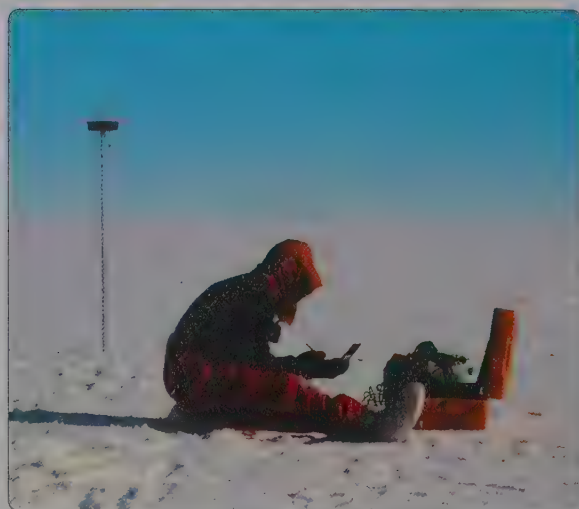
Communications satellites are placed in 'geostationary' orbit above the equator. This means that they move at the same speed as the earth and remain fixed above a single point on the earth's surface. The Global Positioning System (GPS) – seen in use here in Antarctica for monitoring glacier movement – allows accurate position fixing and navigation. Originally developed by the US military, the signals from the satellites now serve hand-held personal and in-car navigation uses, as well as more sophisticated surveying and mapping applications.
