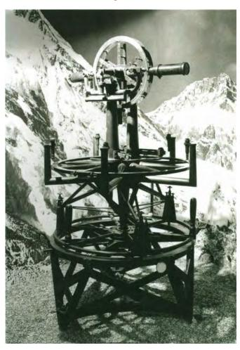
The 'Great' Theodolite was made specially for the Indian survey. Its solidity ensured that the readings were of the highest accuracy.
