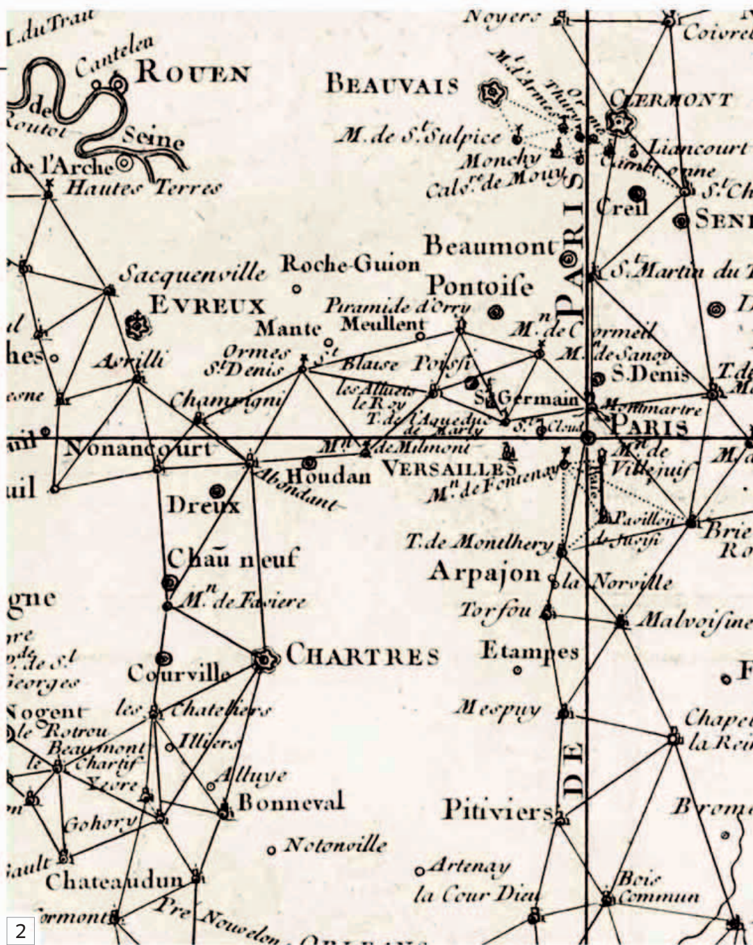
▲ PARIS At the centre of a series of converging triangles stands Paris. The Paris meridian runs directly through both the city and the famous observatory. It is bisected by a perpendicular line from which all the triangles measured by trigonometry originated. On Cassini de Thury's maps, all lines, rather than roads, lead to Paris.
