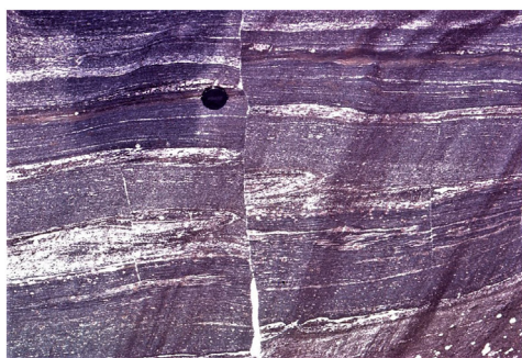
FIGURE 4.1 A fault is a rock fracture across which displacement has occurred. Evidence of the motion on the fault comes from displaced marker layers.
