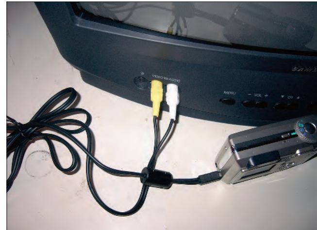
Figure 17-25: Hooking a camera to a TV
