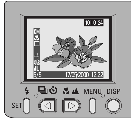
Figure 1-33: An LCD viewfinder allows you to see exactly what the picture will look like
