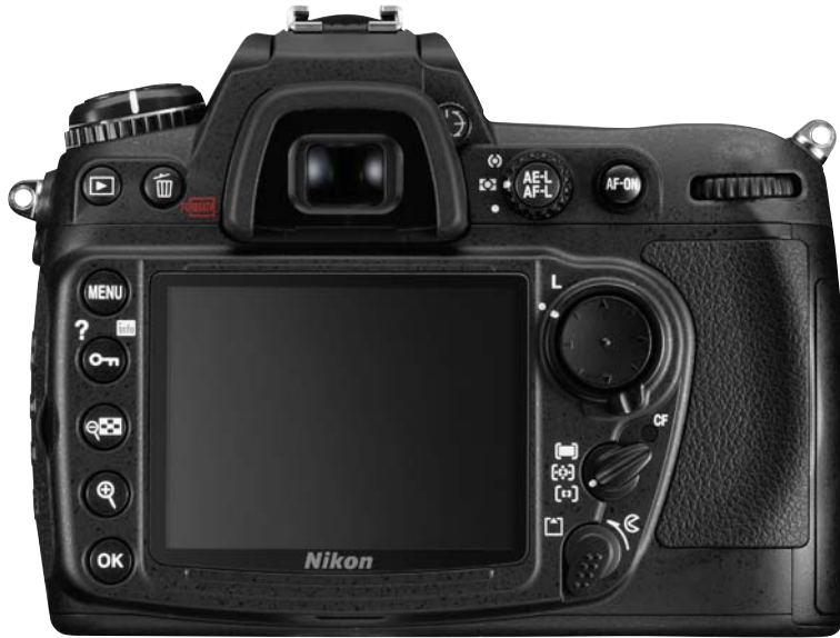
Several manufacturers are now offering large 3.0-inch LCD screens with 922,000 pixels to enable a more accurate preview of image quality
