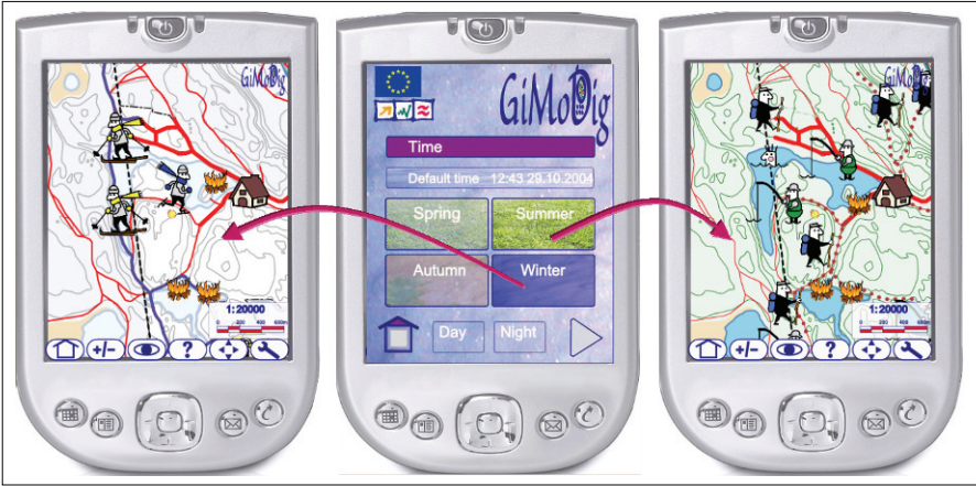
Fig. 10.4. Adaptive mobile maps delivered in real-time from the GiMoDig service. Visualisation adapted for teenagers and according to the time of the year: winter and summer maps
