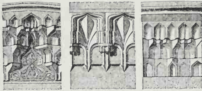
Fig. 14-6. The Koran prohibits in principle the depiction of men and animals in painting or carving. Islamic architecture has consequently developed geometric ornamentation to a very fine art. This is true of the architecture itself as well as the rich decoration. (a.) Examples of stalactite ornamentation, which is used in many variations. (b.) Carved and turned wooden panel fillings.
