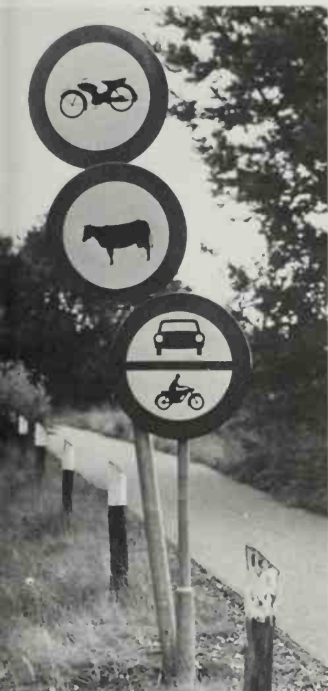
Fig. 3-6. Pictographic traffic signs along a bicycle path. Traffic signs are instantly recognizable to all travelers without further explanation. Sign/symbol language has been most regulated in this particular field, both in form and in color. Geometric forms (circles, triangles, squares) and basic colors (red, blue, yellow) plus black and white are primarily used. In this way these signs acquire an ornamental character.
