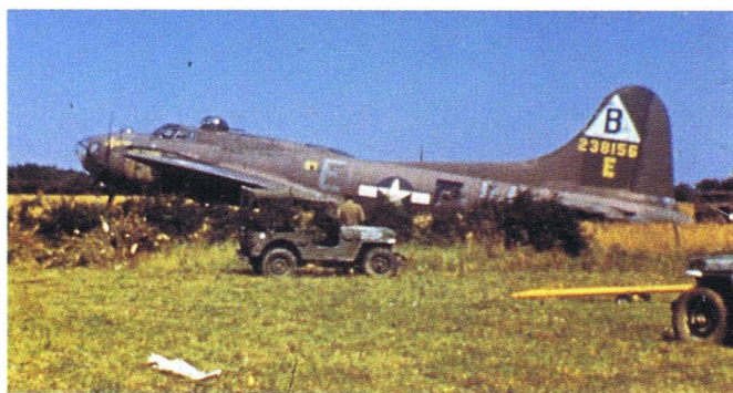
Above: The placement of identification letters on each side of a Fortress with staggered waist gun positions is well illustrated in these two photographs of B-17G 42-38156 JW:E of the 326th Bomb Squadron, 92nd Bomb Group. Mary B overran the runway at Podington early in August 1944, finishing up in a wheatfield. Worthy of note is the darker green of the main fin section and black instead of blue for the letter B. (W. Furniss)
