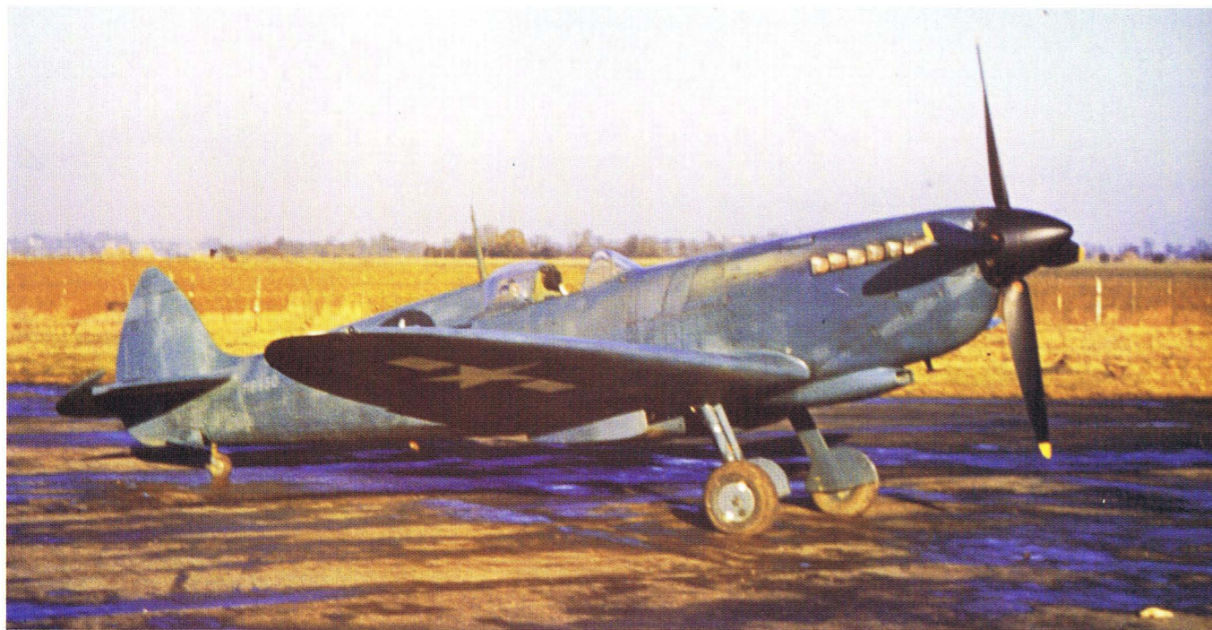
Above: MB950, one of the first Spitfire PR.XIs received by the 7th Photographic Group late in 1943. The serial can be seen on the rear fuselage painted in light grey on the PRU Blue finish. (Robert Astrella)
