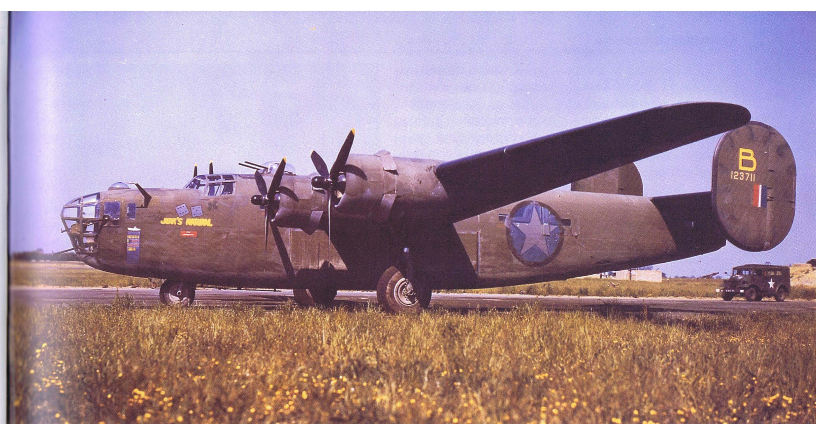
Above: The placement of the individual radio call-letter B above the tail number indicates that this B-24D was assigned to the 93rd Bomb Group's 328th Bomb Squadron. The yellow surround to the dulled cocarde has been painted out with a camouflage green, probably the same shade as used for the blotching round the fin and rudder. The RAF-style fin flash was added when on detached service in North Africa. (USAAF)
