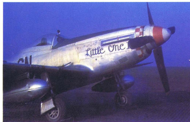
Below: Red and white checkerboard and spinner stripes marked 339th Fighter Group Mustangs. Little One , fitted with 100 US gallon metal drop tanks, was P-51D 44-14622 D7:E of the 503rd Fighter Squadron. (James G. Robinson)
