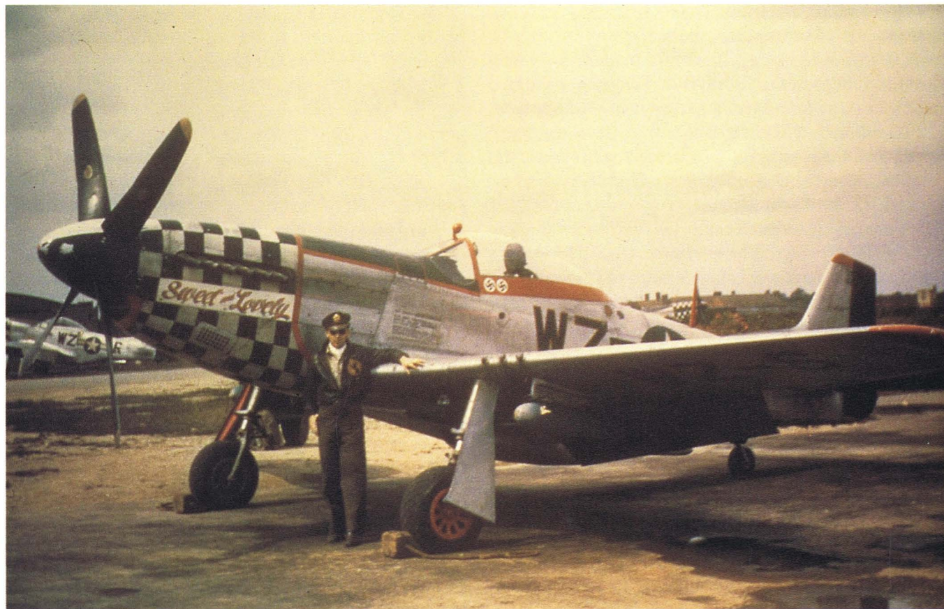
Above: Sweet and Lovely , P-51D 44-72203 WZ:S of the 84th Fighter Squadron, photographed post-VE Day, has the red trim that was used on most Mustangs of the squadron from March 1945. The longitudinal division of the spinner into black and white created a distinct flicker effect when the propeller revolved. (Thomas V. Thain)
