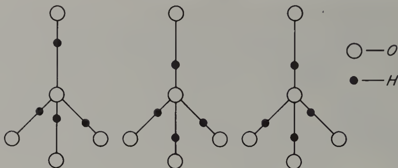
Figure C-19. Three of the six possible environments surrounding an oxygen in ice.
