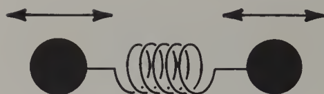
Figure 4-1. Vibration of a diatomic molecule; the spring represents the chemical bonding.
