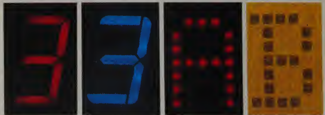
Color Figure 7. Four types of alphanumeric displays based on (a) light-emitting diode (electroluminescence in a semiconductor); (b) vacuum fluorescence (phosphor excited by an electron beam—see also Figure 14-10); (c) helium-neon (gas discharge); and (d) liquid crystal (twisted nematic polarized light rotation).
