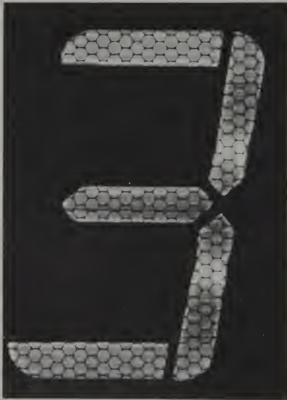
Figure 14-10. Photograph of a vacuum fluorescence display; see also Color Figure 7. Note the hexagonal grid wires and the three horizontal cathode emitter wires.
