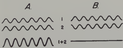
Figure 12-2. Light waves 1 and 2 produce (A) constructive reinforcement if they are in phase or (B) destructive cancellation if they are out of phase.
