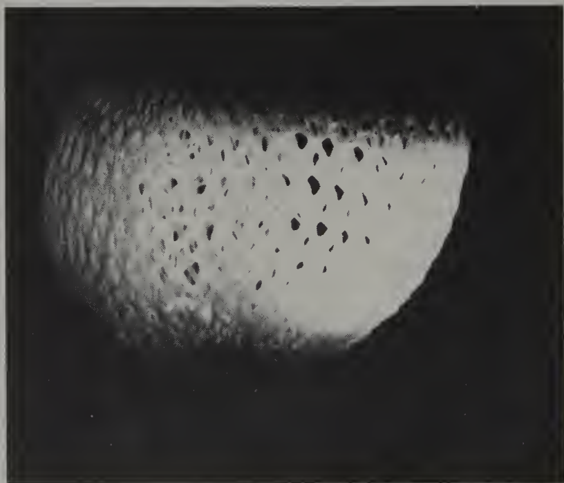
Figure 2-6. Wellsbach mantle in a propane-fueled camping lantern.
