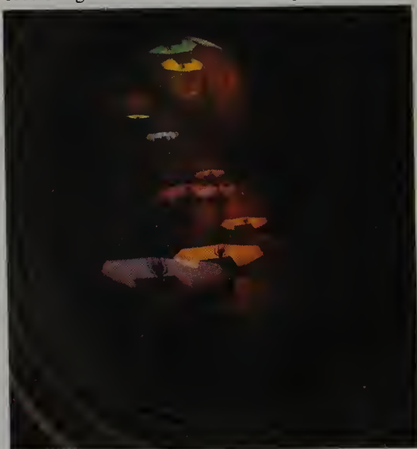
Color Figure 31. Purple reflection (lowest image) of a lamp from the antireflection coating on the top surface of a multielement camera lens; other colored images are derived from multiple reflections.
