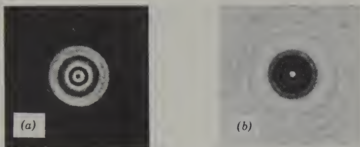
Figure 12-22. Diffraction pattern produced by a point source of light and a small opaque disk (a) or a circular hole in a screen (b).
