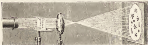
Fig. 22. Dissection by sunlight of a block of ice and its crystalline structure shown.
