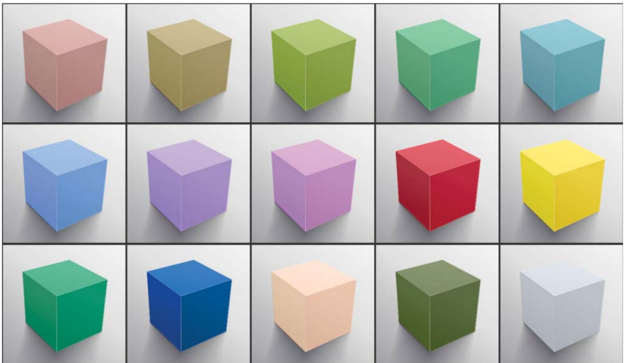
Figure 7.13 Rendered cubes where the top is illuminated by D65, the left-facing side is illuminated by LED B-5, and the right-facing side is illuminated by FL 3.15.
