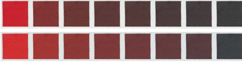
Figure 2.10 Mixtures of red and black paints in either even (top) or cube-root (bottom) increments by weight. The uneven increments result in a more uniform perceptual scale.
