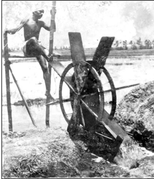
Fig. 8.12 A paddle wheel in operation to lift water from a paddy field into a channel in the Kuttanad area of Kerala!
