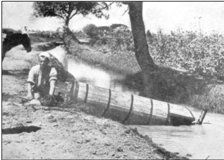
Fig. 8.10 (a) An Archimedian screw (Egyptian screw) being used to lift water from a field channel (minor canal) for irrigation Courtesy: FAO, Rome
