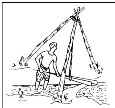
Fig. 8.1 The scoop, with rope and wooden tripod is used to lift water from a shallow stream
