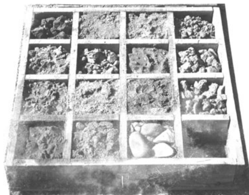
Fig. 5.20 Strata sampling box for well log. The samples obtained from different depths during drilling are collected in different compartments of the sampling box. Note the number tags indicating the ranges in depth from which the samples have been obtained.
