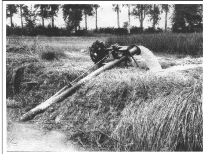
Fig. 12.7 A portable engine operated propeller pump lifting water from a stream to a field channel
