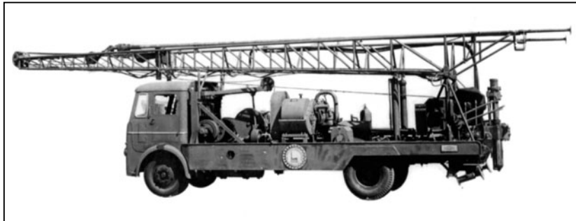
Fig. 5.10 A truck-mounted heavy duty percussion drilling rig in transport position Courtesy: Garlic & Co. Ltd., Mumbai
