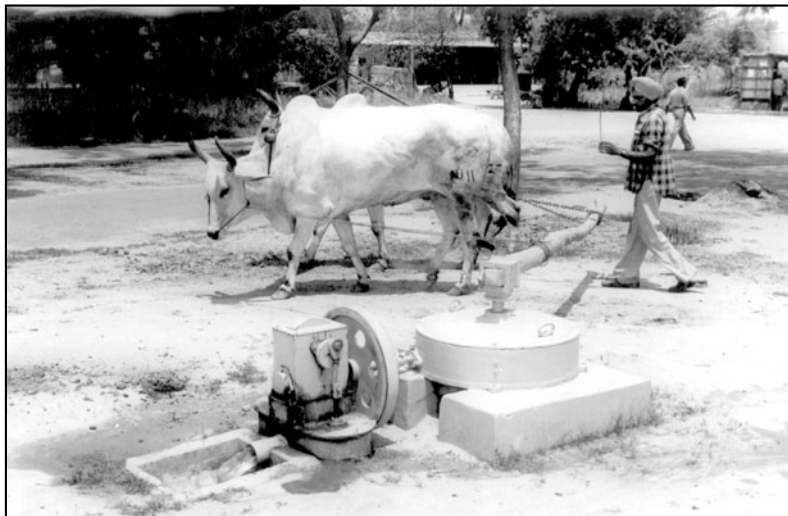
Fig. 8.38(a) An animal operated duplex reciprocating pump in operation on a shallow tube well
