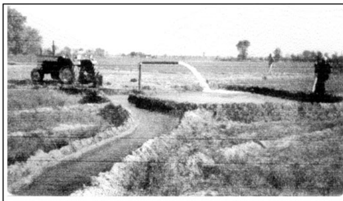
Fig. 10.23 A medium horse power tractor operating a volute centrifugal pump installed to lift water from a shallow tube well. It is an example of using a high power unit for a small load, resulting in heavy loss in mechanical efficiency of the power unit.
