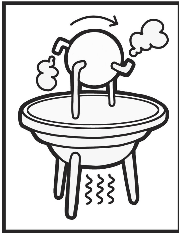
Figure 23: A machine that could've powered the ancient Greek civilization: the aeolipile.
