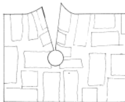
Fig. 12. Cutting the flooring to fit around pipes and radiator legs.
