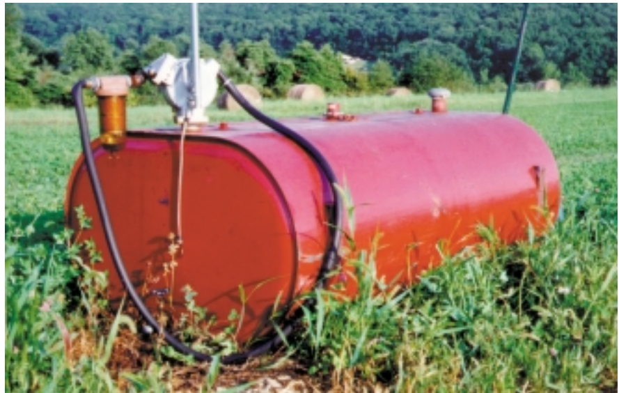
Salvaged 275 gallon horizontal fuel tank with hand fuel pump and filter. This type of pump is suited for all fuels; current use is for diesel fuel..
