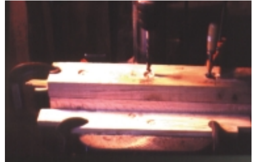
Drilling the hole for the bolt shank
