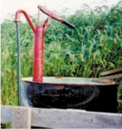
Thirty dollar drum pump mounted on a 55-gallon drum of kerosene. This type of piston pump is not suitable for gasoline.
