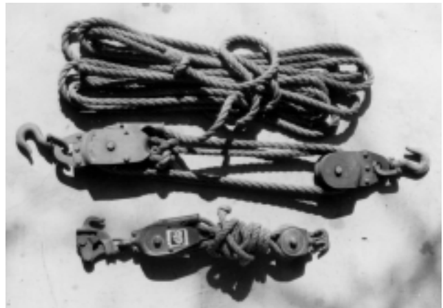
Rope and pulley fence stretchers. Pulling the rope outward at the lever seen on the left-hand pulley locks the rope in place. The operator can then secure the tightened wire in place. The set of stretchers on top has two open hooks.
