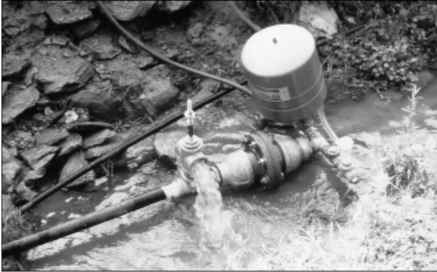
Figure 10: A hydraulic ram is a simple, water-powered pump.
