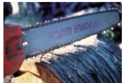
Figure 3. Make sure the saw's bark-dog is touching the round before the moving chain touches the wood.
