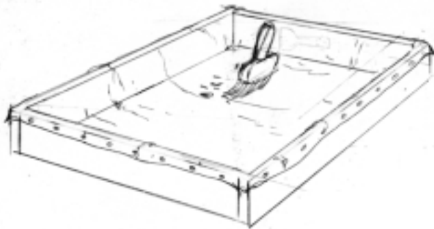
Figure 21. A wooden box may be lined with heavily painted cloth and used as a wading pool. Allow the cloth to overlap over the edges. Tack or staple in place before painting.
