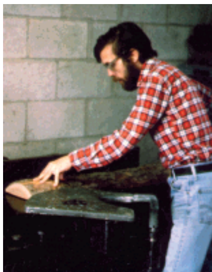
The author surfaces a cherry slab board on his antique 16-inch jointer.
