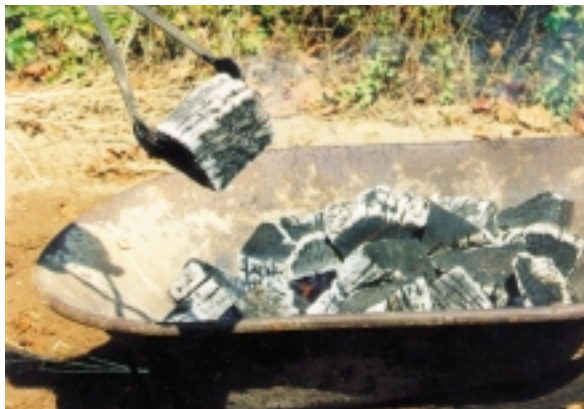
As the charcoal briquettes are fully burned on the outside, use metal tongs to place them in a second container, or drop the pieces into a fire pit where carbonizing action occurs.
