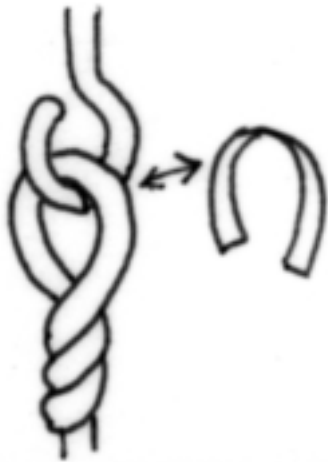
Figure 14. When hanging swings from metal eyebolts, using eyes designed for splices in cable allows rope to hold up much longer.
