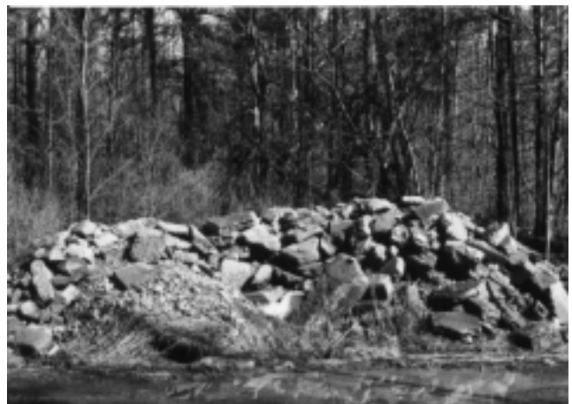
This is the concrete block used to form the base layer of the road
