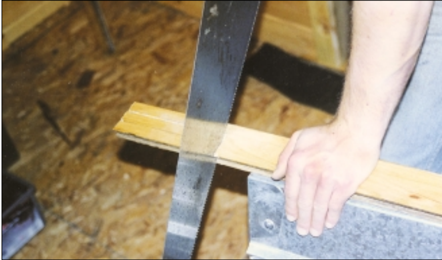
Use a handsaw when cutting the oak in order to prevent end-splintering.
