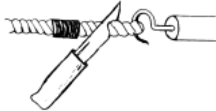
Figure 8. Whip or tape the end of the rope, about an inch back, then cut it free
