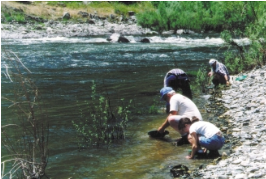
Panning is the basic gold extracting method but usually is employed to find “color” only. Sluices and powered units are more efficient.
