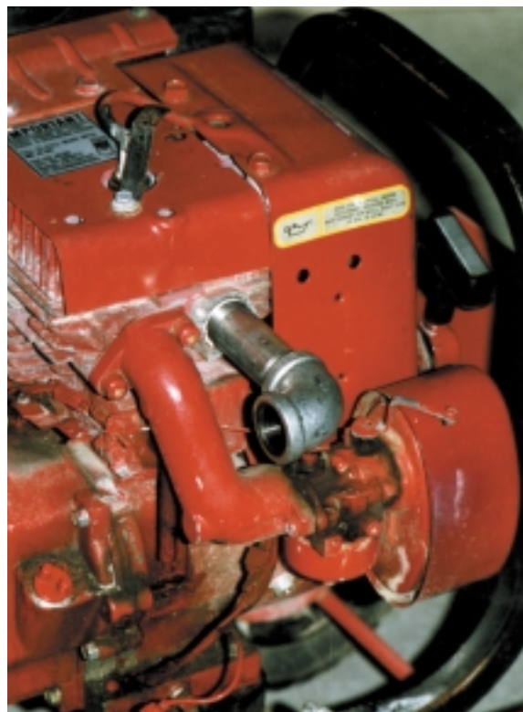
In this picture, you can see where I threaded an extra nipple into the engine. I used Teflon plumbing tape to seal the threads. The 90-degree elbow is where I will attach the nipple/connector/exhaust-pipe assembly. The muffler then slips over the assembly.
