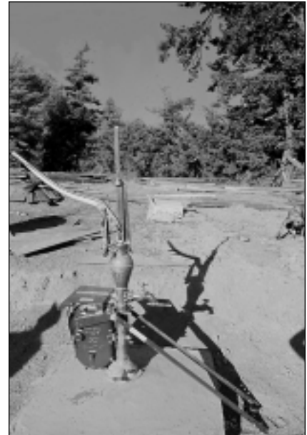
Figure 8: A pump jack mounted on a pump standard offers hand and powered pumping.
