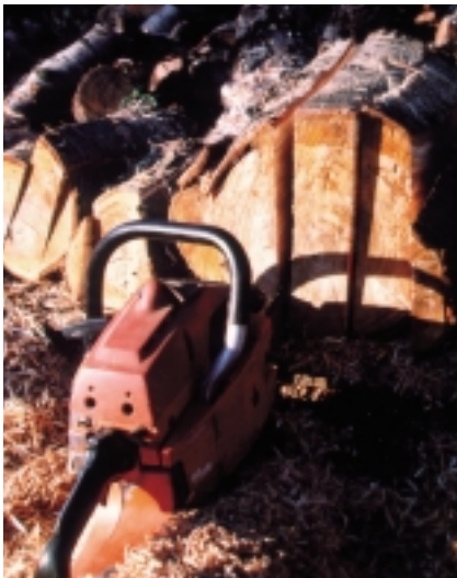
Figure 2. Making little slabs out of big rounds. If a round needs more than one cut, make the side cuts first.
