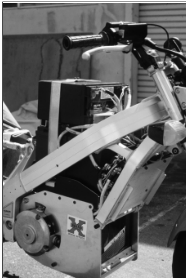
Four 12V sealed lead-acid batteries just fit under the tank in the Hawk.
