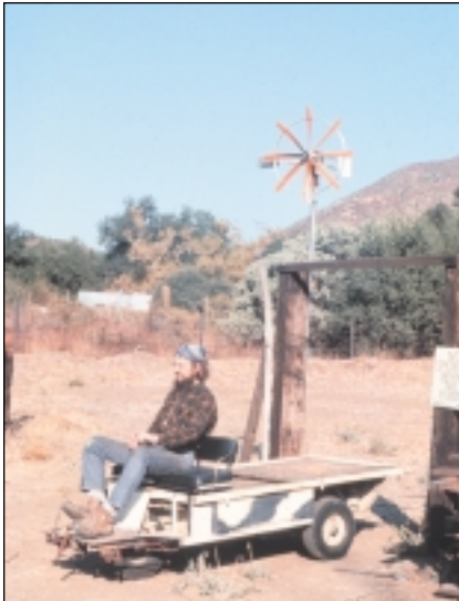
Wind-generated electricity was used to recharge Ox.
