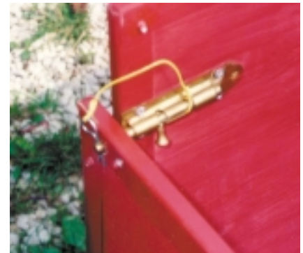
Closeup of the sliding doorbolt with a clip used to secure the front end gate to the cart panel
