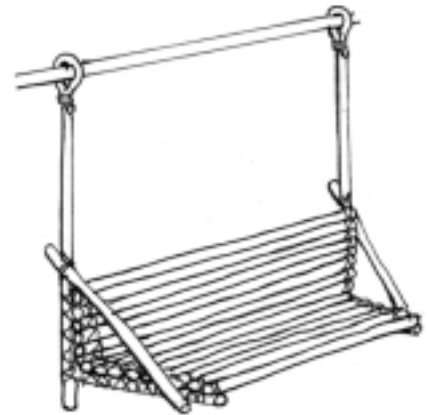
Figure 11. Lash poles in place for seat, back, and braces.
