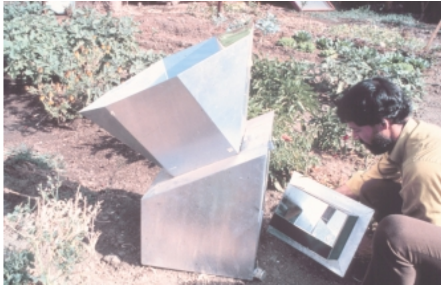
Solar cookers achieve 250-350 degrees during operation.
