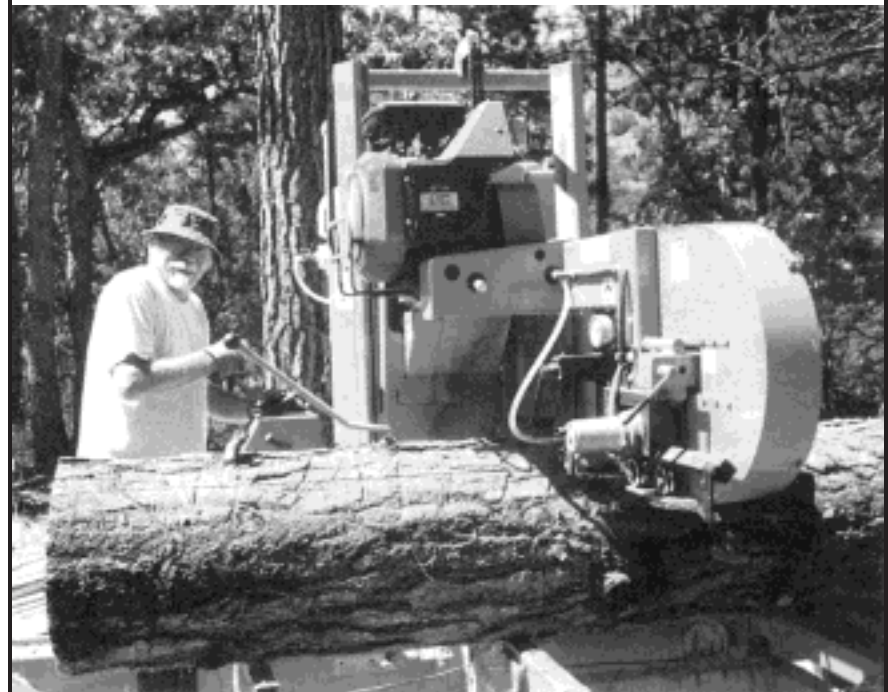
Rich Perrigo of Montague, California, uses a Wood-Mizer sawmill to cut a pine log into timber.
