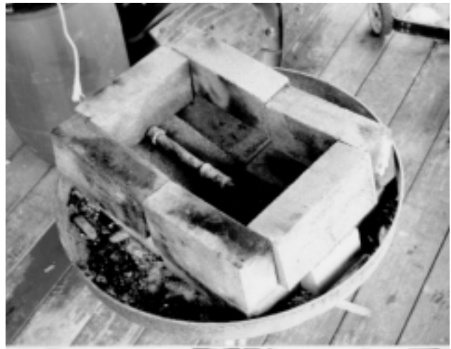
The portable forge, made from an old charcoal grill, fire brick, and iron pipe.
