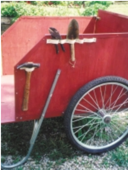
Detail showing tool loops and metal edging attached by pop-rivets
