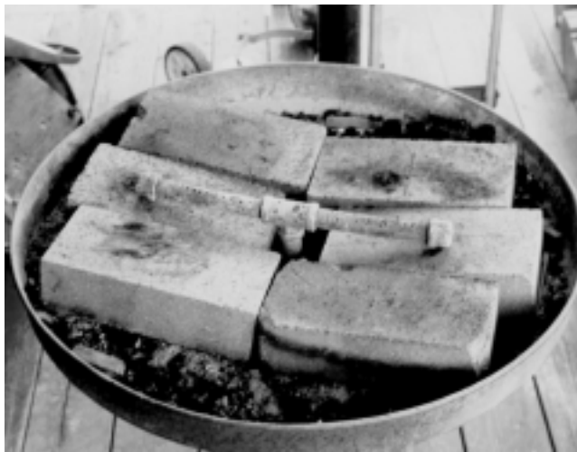
Placement of the bottom bricks and tuyere
