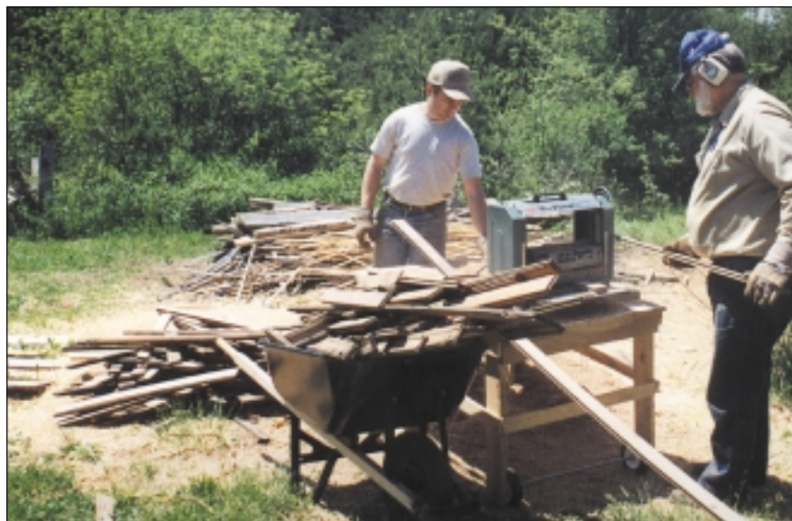
To clean off old stains or varnishes, use a planer set so that the blades barely touch the wood.
