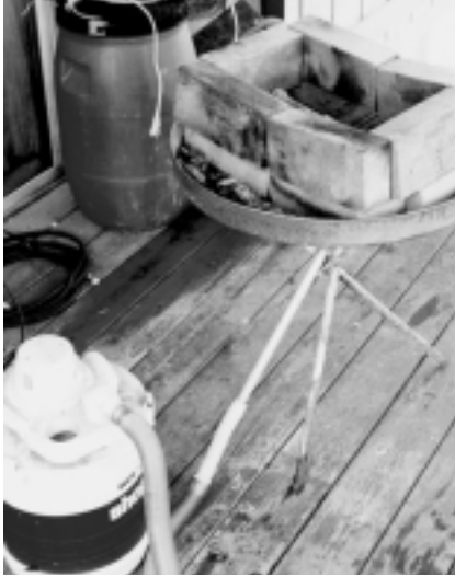
Assembled forge with shop-vac
