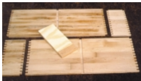
Figure 2. Parts making up the two-drawer chest
