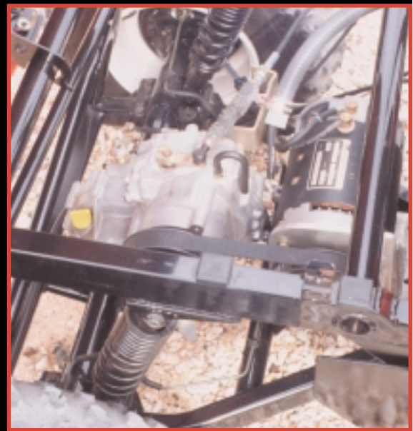
A gearbelt delivers motor power to the stock transmission, eliminating the less efficient infinite ratio drive unit.
