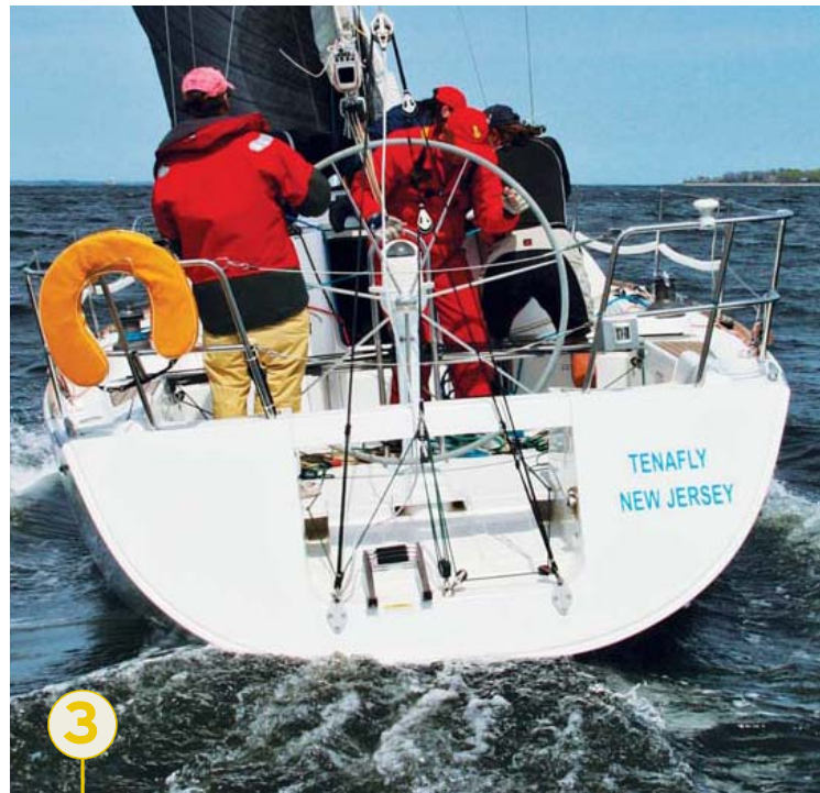
PHOTO 3: Once inside the lifelines, the jib is trimmed to 80 percent, marks on the sheet help this happen on every tack. The lead is in its forward position to power up the top of the jib.
