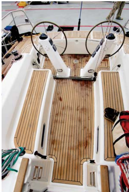
In the Salona 45's salon (above), the galley and the settee flank a bench seat that's easily removed to check the keel bolts and the bilge. The cockpit, shown with the twin-wheel option, is a good working area for a racing crew.
