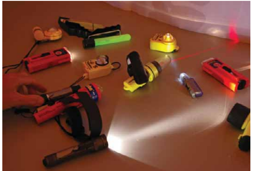
A variety of lights were tested during the COB Symposium. One of the brightest was the Surefire flashlight (bottom), which is designed for use by police and military forces.
