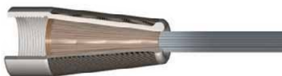
Element C6 end fittings (left and above) are composed of pultruded carbon rods embedded in epoxy cones. Element C6 Plus, which is continuous, needs no fittings on the spreader tips (top) of the Carroll Marine 60 Numbers.
