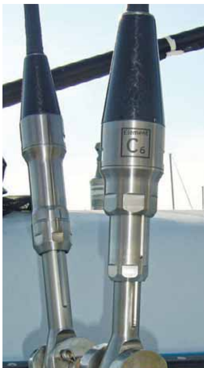
Element C6 end fittings (left and above) are composed of pultruded carbon rods embedded in epoxy cones. Element C6 Plus, which is continuous, needs no fittings on the spreader tips (top) of the Carroll Marine 60 Numbers.
