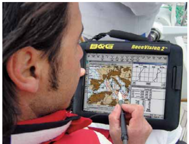
THE B&G RACEVISION 2 is a stand-alone tablet computer pre-loaded with B&G's Deckman for Windows software.
