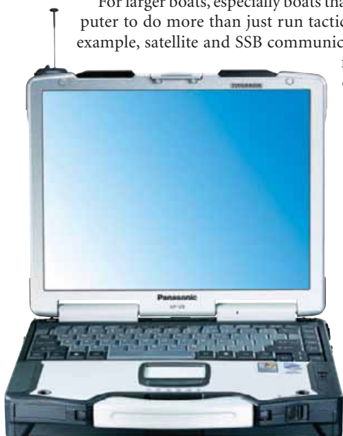
THE PANASONIC TOUGHBOOK's hard drive is encased in a shock-absorbing polymer.
