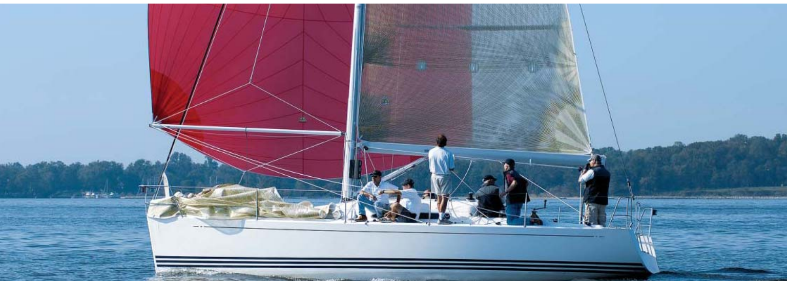
Future X-35 One Design crews will enjoy stanchions located well outboard, a rounded hull to deck joint, and the absence of toerails aft of the mast.
