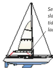
First reef taken in – slab is often left loose
