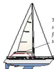
Short battens must be used for in-boom roller reefing
