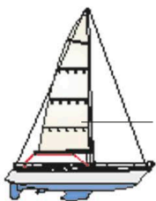
Modern slab reefing is used on fully battened sails
