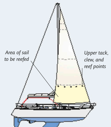
Second reef slab is usually tied with a lacing line
