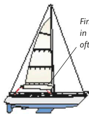
Modern slab reefing is used on fully battened sails
