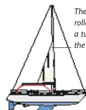
The amount reefed can vary from one to several rolls
