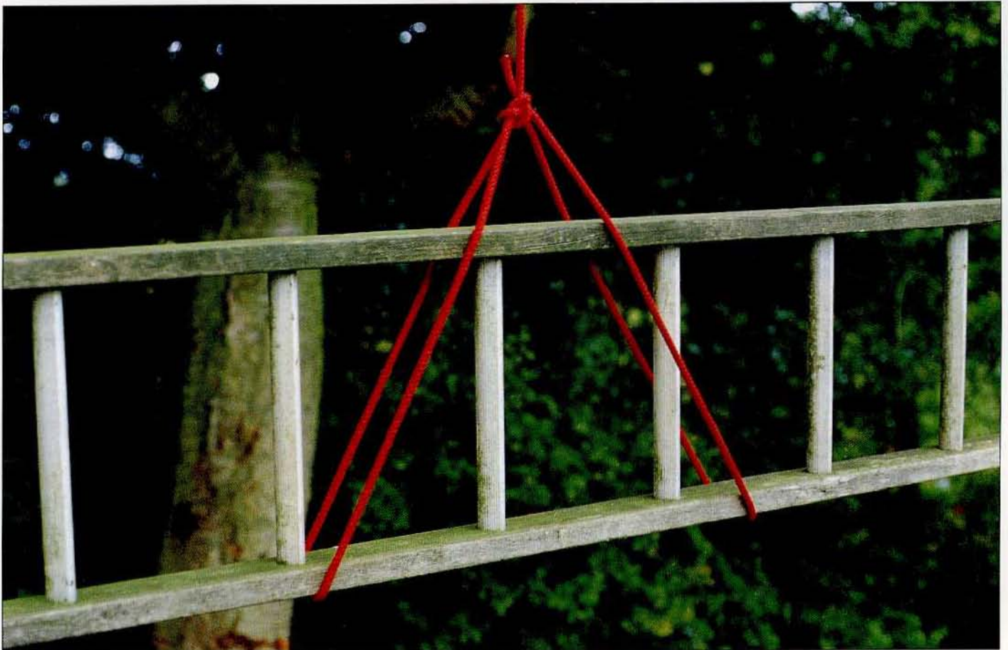
The Spanish bowline is a versatile knot which is used in many situations including rescuing people from the sea and hoisting objects in a horizontal position.
