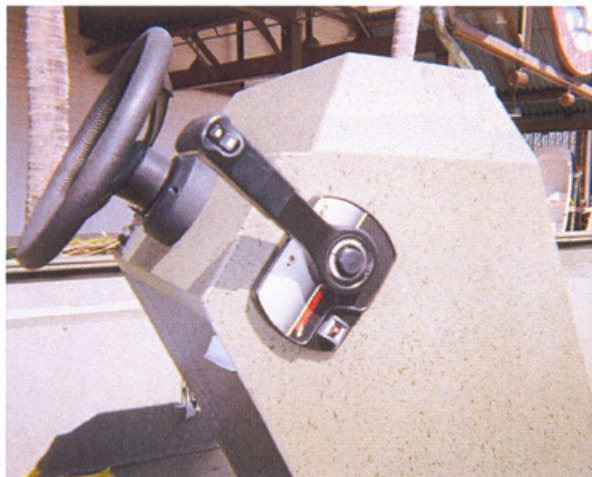
Throttle Control / Transmission Control: Selects forward, neutral and reverse gears and controls propeller speed.
