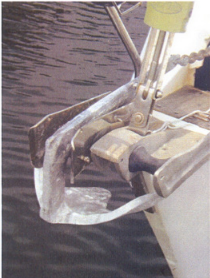
Anchor: A device attached to rope or chain which is lowered to the seabed to hold a vessel in place.
