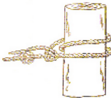
Round Turn and Two Half Hitches
