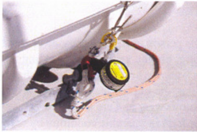
Hydrostatic Release attached to the liferaft
