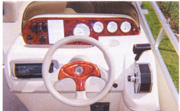
Console: Steering console, instrumentation and throttle control
