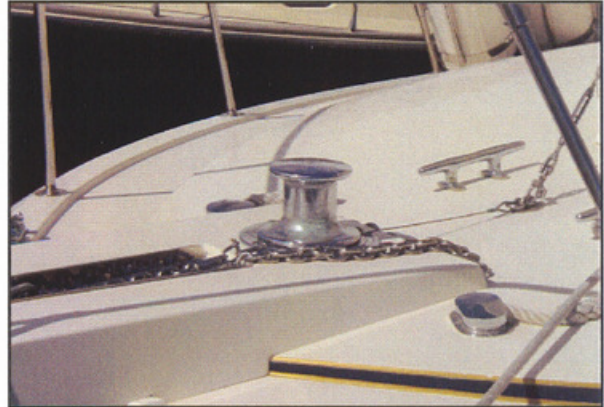
Windlass: A winch which is positioned on the fore-deck and used for hauling in anchor chain and rope.
