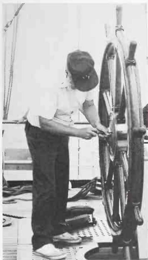
Eagle's main wheel about to be dismantled for repair and adjustment of the main shaft. Meanwhile, the ship's steering is transferred aft to the auxiliary coffin wheel on the poop deck. In the North Atlantic, summer 1985. (U.S. Coast Guard photo by Doug Bandos)
