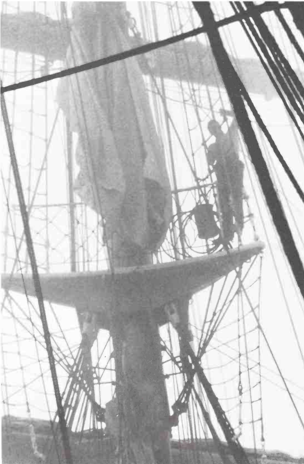
A foggy day finds a crew member slushing down Eagle's cable rigging. A mixture of oils and solvent is regularly applied to standing rigging, penetrating to its heart and protecting it from the ravages of the salt-water environment. (Peter Geisser photo)
