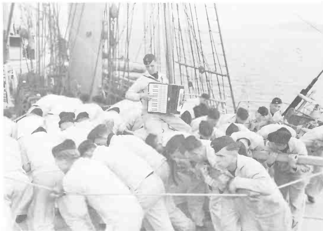
Horst Wessel crew members singing sea-chanteys as they bring up the anchor chain in the Baltic Sea off Danzig (now Gdansk), spring 1944. Two-and-a-half rotations of the capstan were required to raise the chain one meter; at times it was as deep as 270 meters. Note 20 mm gun at right. (Courtesy Tido Holtkamp)
