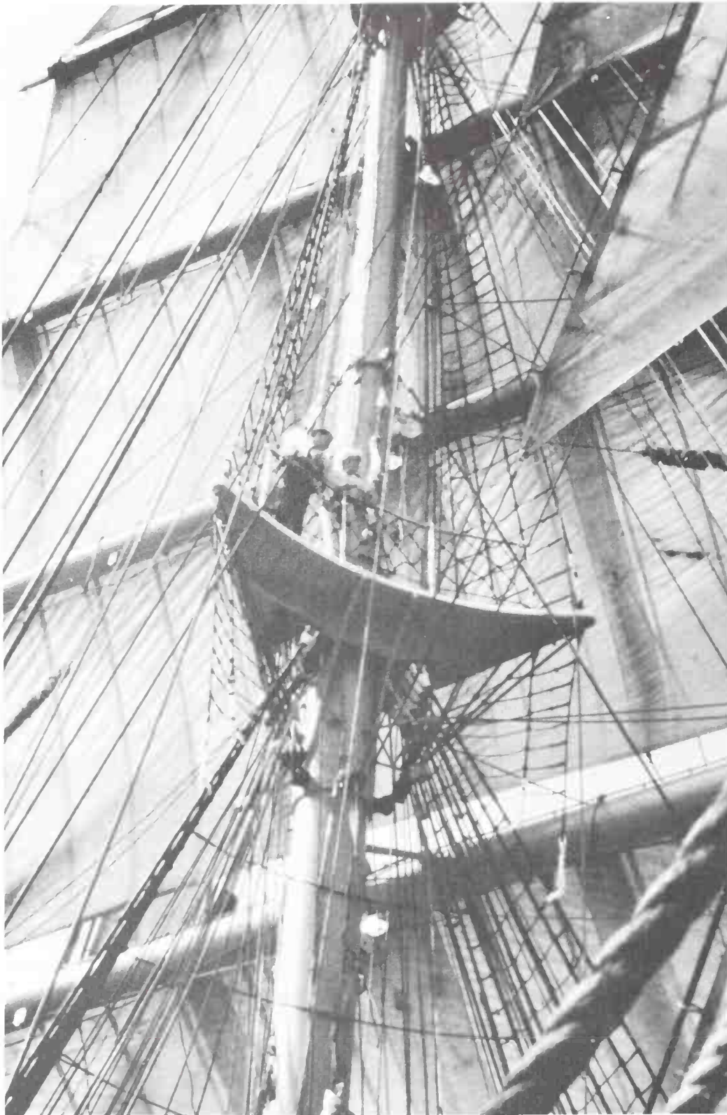
Under full sail, the mainmast presents a wall of canvas. From bottom to top, the square sails are the main course, the lower and upper topsails, the royal, and the topgallant. A cadet in the "tops" works on rigging maintenance. (Peter Geisser photo)
